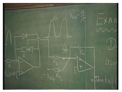
So, in our case, we want this peak to be equal to 100 millivolts. So, V p is equal to 100 millivolts. So, that is equal to pi into V reference. So, we have V reference equal to 100 millivolts divided by pi millivolt. How much? 31 point 8. So, that is the V reference that you have to connect here in order to make the peak voltage equal to 100 millivolts, constant.
