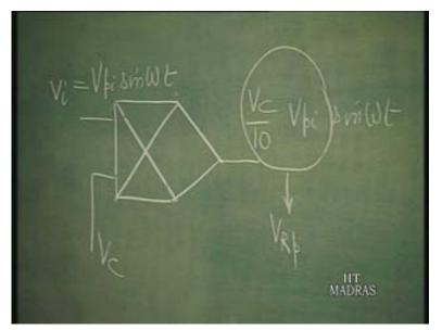
Now, what is the range in which this A G C system will work? Let us see. V c utmost can be equal to 10 volts. So, when V c is 10 volts, V p i has to be equal to V R p.
