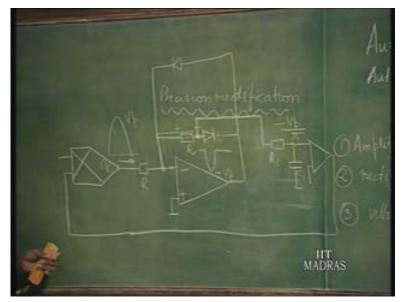
So, I would leave it as an exercise for you to find out what should be the polarity here; should it be negative or positive so that the entire feedback system becomes negative feedback system. How do you find out that? Assume that this amplitude is growing...this becomes more negative than this. It has been compared with negative voltage. If it becomes more negative, what should happen to this voltage such that the gain is reduced?
