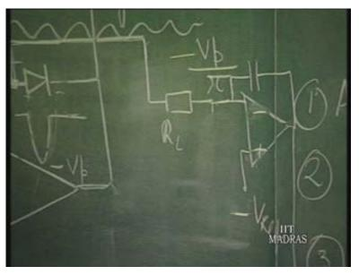
Another variation of this is, instead of using minus V reference and connecting it here, I can remove this and connect it here and make this plus V reference and this also R l.
