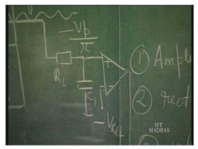
So, you can make it work actually by putting here negative and positive and assuming that this is working only for negative voltage here. So, then I can put this capacitor as a feedback capacitor. This is called Miller effect. That also I have discussed earlier. So, this capacitor appears as a huge capacitor at this end point. That is possible only if this is negative because this tries to give negative feedback. So, this controller now becomes this way.
