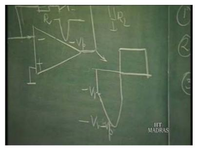
Only when it is going positive, the output is coming as negative at this point. So, this is the point at which output is going to be taken. So, please remember that both diodes are necessary. If it is positive half you want to select, you will invert the diode here and put the other diode in the other direction. So, this is the circuit for a half wave rectifier, precision rectifier.
