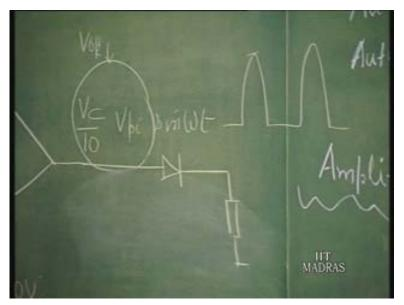
Let us say, after generating this rectifier wave form, I want to filter this. How can I do that? That can be done by putting a low pass filter. This is the arrangement of the low pass filter.
