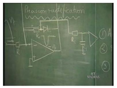
Please see here that, now I have obtained the negative voltage as the peak. So, it will be...this voltage will be minus V p divided by pi. So, I can compare it with...again with V reference which is negative because this voltage will always be negative. So, I have to have V reference which is negative and appropriately apply the feedback here so that this system now functions satisfactorily. Is it clear?
