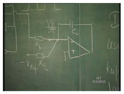
Let us consider this. So, this is the V i which is V p i sin Omega t. So here, we have V c V p i sin Omega t divided by 10 as the output. The V c can be positive or negative. We want to see for which one it is negative feedback. That is all, because all the other things are frozen here. So, we have now the choice to see whether it is positive feedback or negative feedback, for positive or negative voltage. Let us see.
