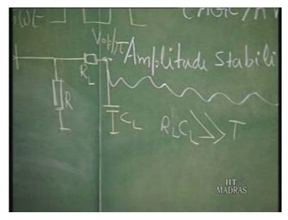
In such a situation, the D C output voltage here is going to be V naught p by pi and this D C voltage can be used assuming that the diode is an ideal diode. We have got this much information, that the D C voltage is V naught p by pi. Let us see. If this increases, this voltage is going to increase. So, this information gives straightaway the fact that I have to decrease the gain.
