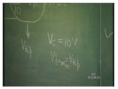
That is the range in which this system will work. That is the maximum gain you can give from your amplifier. So, the maximum gain times the minimum voltage should be equal to whatever value you get. That is number one.
