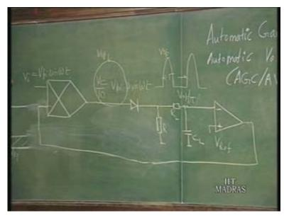
So, we have now built a system which is called automatic gain control or automatic volume control. This rectifier filter combination will measure the peak value voltage and compare it with V reference and have the control voltage controlled in such a manner that the gain is decreased if the amplitude is increasing, and the gain is increased if the amplitude is decreasing.
