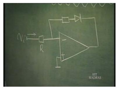
So, as long as V i is greater than zero, this current is positive and the diode automatically conducts. Why? Let us try to understand. If the diode does not conduct, then this is an open circuit. If this is an open circuit, this voltage will directly appear here and this voltage will try to go to negative saturation. That means this diode will be forced to conduct because this voltage will go towards negative value.
