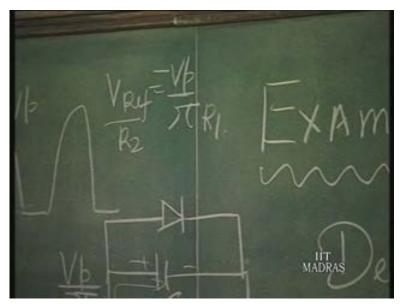
So, minus V reference divided by R 2 plus V p by pi divided by R 1 is equal to zero. So, this is the current equation. In general therefore, this could be made different. R 2 can be made different from R 1. Let us say this equation is what is important.
