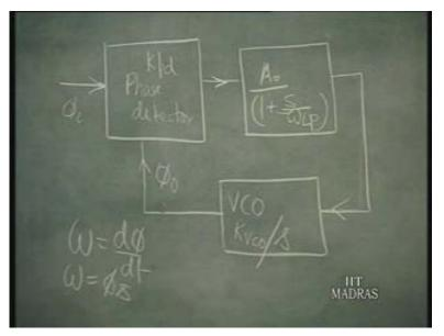
Let us now see how this is going to respond. phi i minus phi naught is the phase difference and Kpd into that is the D C voltage here or low frequency voltage here and that is getting amplified by A naught divided by 1 plus S by Omega L p.
