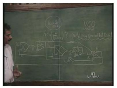
In this particular circuit, you... if this is V p sin Omega T, this output is going to be V p cos Omega T because this is integrator; and if this is V p sin Omega T, this is going to be V p cos Omega T and therefore we can square these using multipliers and simply add. Therefore, the way to build this circuit is you just take these outputs, square these and add. Adding can be done by using just a resistive network like this.
