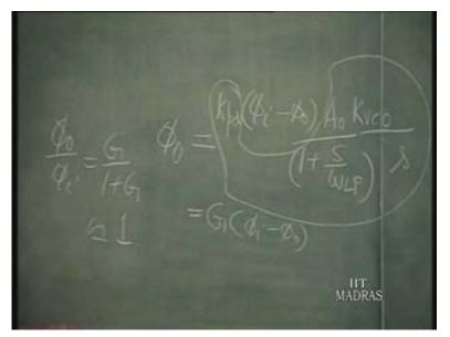
Now, what is G? The loop gain here is nothing but Kpd Kvco into A naught. So, that divided by S into 1 plus S by Omega Lp. This factor, which is independent of frequency, is called the D C loop gain of the...this K l, which is nothing but...you go through this...Kpd, A naught, Kvco, all the sensitivity factor products. You call this as D C loop gain. So, this is going to be equal to K l divided by s into 1 plus by s by Omega L p.
