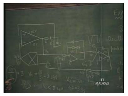
Further amplitude build-up will not occur because now the amplitude is going to be such that V reference is going to be equal to V p naught by pi for this kind of relationship. And therefore, if we want output voltage peak amplitude of 10 volts; that divided by pi should be the voltage reference that you have to connect here. 10 by pi here. This is one answer. What is that equal to? About 3 point... 3 point 18 volt.
