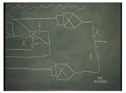
If this is done, this is V p sine Omega T. This is V p cos Omega T. So, what will be getting here will be V p squared by 10 divided by half, because of this resistive attenuator, into sine squared Omega T plus cos squared Omega T, which is constant.
