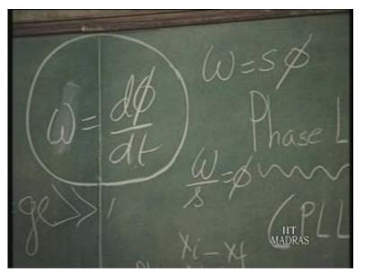
So, if I have frequency, I can say that if the frequency output is given to a phase detector, it will respond to phase change. Therefore, the basic building blocks of a phase locked loop will be a phase detector, a VCO and an amplifier; and it should respond to only average here because D C, I said. So, amplifier with a low pass filter.
