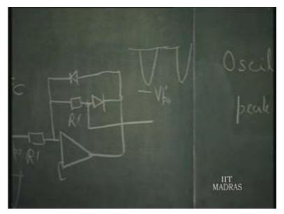
And then we put the low pass filter which is now converted into an integrator. We have seen this, the Miller effect and all comes into picture; R double dash. And we will put a voltage reference here. Since this is negative, it will give a negative average; voltage reference should be positive. So, at the time of starting, this has no voltage here; amplitude has not built up. So, there is V reference which is positive. This will be driven to negative saturation.
