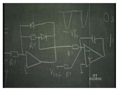
Let us say, the supply voltage is plus 15, minus 15 for this op-amp. So, it will go to minus 15 volts here. So, this minus 15 volts has to be converted into something suitable so that V c becomes equal to your 3 volts so that it can start oscillating. So, we will put an attenuator here. So, we will connect here plus 15 volts let us say. So, this voltage becomes 3 volts initially. That means this Alpha R, this is 1 minus Alpha times R, an attenuator.
