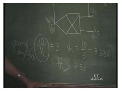
That is, the gain should be greater than 3. Let us say therefore, V c should be less than 3 point 33 volts. Gain should be greater than 3 and therefore V c should be less than 3 point 33 volts.
