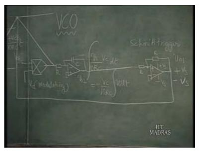
So, this circuit can be also converted into its transistor counterpart wherein this portion is going to be replaced by a voltage controlled integrator. That means you will have a voltage controlled current source driving a capacitor. That is all. And a transistor I Schmitt trigger; but the basic circuit is essentially this.
