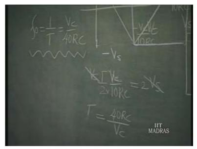
So, this particular thing is a nice voltage controlled oscillator, linear, but it uses only one multiplier. It does not require any amplitude stabilization scheme because already the amplitude gets neatly stabilized at plus V s and minus V s and this rate of rise and rate of fall become same; equal to minus V c V s by 10 R C and plus V c V s by 10 R C, respectively.
