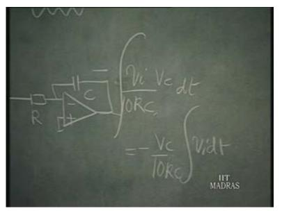
So now, we will do the time domain analysis rather than Laplace because this is going to be connected to a Schmitt trigger which is going to be a regenerative negative feedback circuit that we have discussed earlier. Let us say, this is now plus, positive feedback, local positive feedback is there; and therefore this is R. This is, let us say R and then this is now connected to the input. Let us see what happens?
