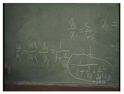
This is an important property of phase lock loop; output frequency will be exactly equal to input frequency.
