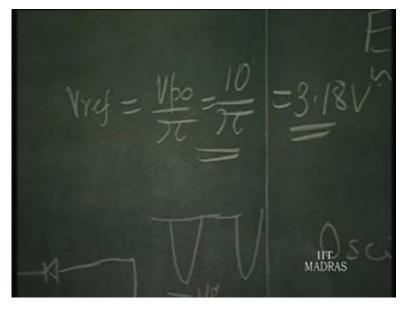
So, if you apply that voltage here, then the amplitude is automatically going to be adjusted to exactly 10 volts peak. Now, one...only one thing is left out. The frequency f naught is equal to 1 by 2 pi R c. That is required to be 1 Kilo hertz. So, 10 to power 3 hertz. So, R c is going to be equal to 1 over 2 pi into 10 to power 3.
