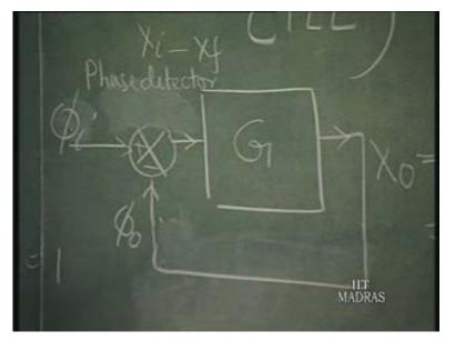
That means, a phase detector is something that...when phase is given as the input, phase difference is given as the input, it will give a D C output corresponding to the phase difference. This D C output is amplified and this output of the amplifier has to be converted again into phase.
