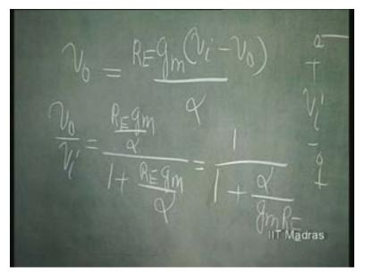
Alpha is very nearly equal to 1; g m into R E is a huge value supposedly and therefore this is going to be very nearly equal to 1.
