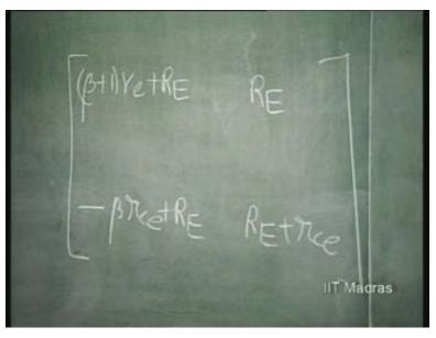
So, this is composite z parameter of this feedback structure which is nothing but this.
