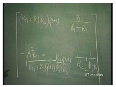
These are the open circuit parameters; these are the short circuit parameters. And, you can see that amplifier does not contribute to the feedback. Only the passive network contributes to the feedback. Here, this is the output conductance of the amplifier. This is the conductance of the feedback network.
