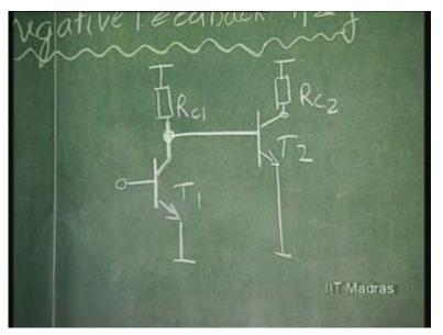
What is h? It is series at the input and shunt at the output. g feedback is shunt at the input and series at the output. h feedback is adopted in order to obtain a voltage control voltage source. So, h feedback is adopted for an idealization towards voltage control voltage source. g feedback for an idealization towards current control current source.
