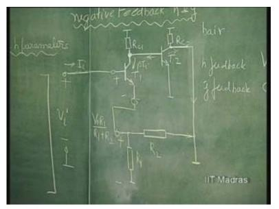
So, minus R 1 by R 1 plus R 2 times Beta plus 1 times I i. So, this contribution is due to the feedback network. This contribution is due to the amplifier. It is dominant. You can see Beta squared appearing here. So, this may be negligible, because there is an attenuation and just only Beta plus 1 here.
