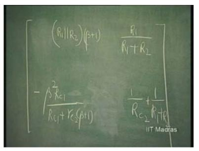
So, minus Beta square into R 1 by R 1 plus R 2 into R c 1 by R c 1 plus r e 2 Beta plus 1. That divided by R 1 parallel R 2 into Beta plus 1. This into 1 over R c 2; 1 over R 1 plus R 2. As long as this is much greater than 1, there is good negative feedback here; and therefore, it is a good negative feedback structure. And therefore, it will result in a good voltage control voltage source.
