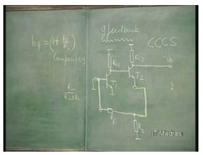
And what happens to the input impedance? It comes down. Output impedance should go up. Or, in the h parameter, h i, h r and h o, all these three things should go towards zero. Only h f should get stabilized at a value of 1 plus R 1 over R 2.
