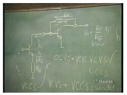
So suppose R f is 10 K and R E is 1 K. You are now designing a nice voltage control voltage source of gain equal to 10 without taking request to the h feedback with the pair that we had earlier discussed. Similarly, you say, I want a current control current source; not this. Then, what you do is simply put this first. R F. So, put this first. Current control voltage source put first and then you put this later.
