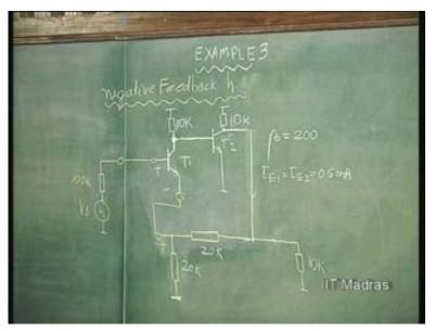
Now we have a source with 100 K, source impedance, and a load of 10 K. So, this is the practical situation. This circuit is the A C picture of the feedback amplifier network. Beta of the transistor equal to 200; and these two transistors are made to operate at a current of point 5 milliampere with the resultant effect r e 1 equal to r e 2 equally, to roughly equal to, 50 ohms. That is, 25 divided by point 5 ohms. So, 50 ohms...
