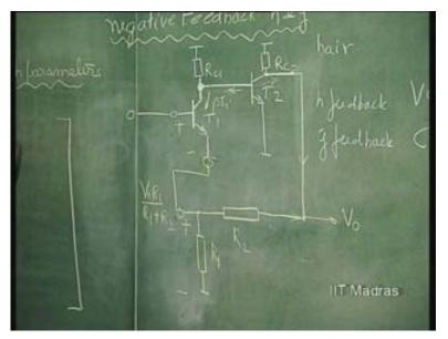
So, this is h r. The fedback voltage from output to input when the input is open is simply R 1 by R 1 plus R 2 times... So, this is h r. Very simple. Then, the output impedance is V naught by I naught here. So, there is R c 2 shunting this. Nothing is happening. This is zero, this is zero. So, these things are ineffective.
