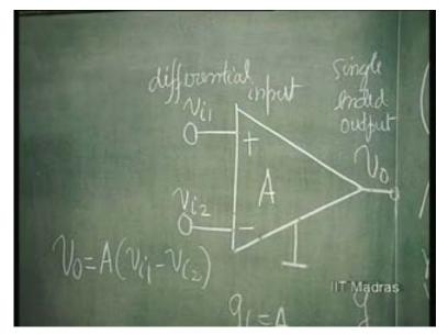
So, if you consider first that only the forward transfer parameter is con ... high, rest of the things are all going to be zero, zero, zero, then, we can indicate that V i 1 minus V i 2 always becomes equal to V naught by A. This is an important principle I am trying to discuss. A is tending towards infinity; which means in an op amp, we can pronounce a statement which is always valid.
