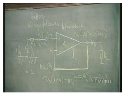
So, this is an important application of voltage follower which is also called buffer stage. Now, if you use the nullator-norator concept, then we do not have to go through this. A is definitely infinity and it is to be indicated very clearly that all this thing is irrelevant, if output is finite; then, this should be equal to this. So, this is already equal to V i. So, V naught is equal to V i; that can be concluded without any problem at all.
