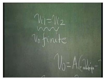
This is an important principle that is used in diagnosing any fault associated with an operational amplifier. That, what it means is, this voltage is same as this voltage. That means this voltage difference is zero; or, this circuit is not drawing any current.
