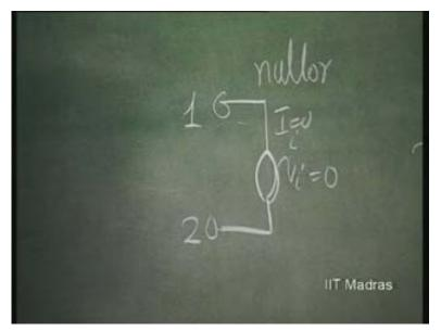
And, of course, at the output... output can be anything finite. So, it can have any voltage and any current. So, this is a norator. So this is the simplest equivalent circuit in terms of nullator-norator, for an operational amplifier of this type. We have already discussed this nullator-norator concept earlier in equivalent circuit.
