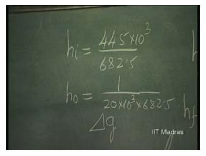
So, the output resistance, R out is going to be 20 into 682 point 5 K; or going... it is going to be of the order of mega ohms.
