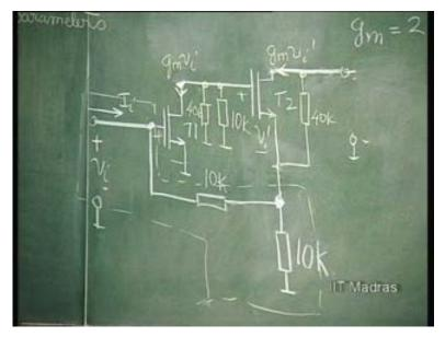
So, this resistance that comes is simply equal to... g i is equal to 1 over 10 K plus 10 K. That is, 20 K, simply. That of the amplifier... g i amplifier is zero; the conductance, input conductance of the amplifier is zero; or input impedance is infinity, in the case of MOSFET. Otherwise, that would have been added to it.
