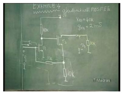
So, in this problem, the actual load is not given; just the R D 2 has been given as 10 K. That has been put here. So now, the current is common to the load, the amplifier and the feedback network. This is how it should look.
