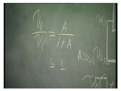
So, voltage, output voltage, will be following input voltage irrespective of the load. Whatever I connect here, it does not matter. So, if I have a source here R s and then V s, we can see that there is no current drawn here and therefore V i is going to be same as V s, irrespective of the value of R s because there is no current in R s; and V naught is going to be same as V i. Therefore, V naught is going to be same as V s. So, this is called a buffer stage.
