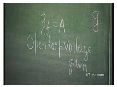
So, V naught is going to be A times... this is called non-inverting amplifier terminal; this is called inverting terminal. So, V i 1 minus V i 2; it is always referred to single ended output. That means, one is... one end of the source is grounded; other end is giving you an output V naught equal to A times V i 1 minus V i 2. So, differential input, single ended output, we are talking of.
