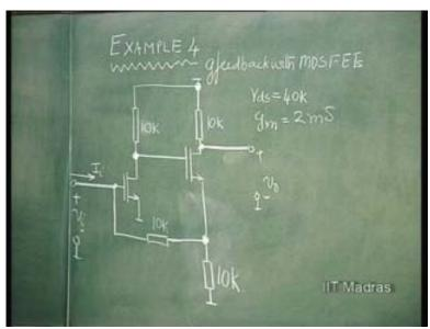
So, we have MOSFET T 1 amplifier cascaded to MOSFET T 2. Actually, this is, this was originally grounded and we wanted g feedback. So, we put the network shunt at the input and series at the output. So we connected it in series. So, this is the feedback network that comes into picture here; coming in series at the output and in shunt at the input.
