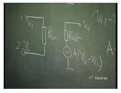
So, this is the equivalent circuit of the operational amplifier. Normally, the order of input impedance for typical operational amplifiers, which are general purpose operation... For example, popular one is 741 or 747 op amp. R in is of the order of 1 mega ohm. R out is of the order of about say, 50 ohms. A naught, that is D C gain here, is of the order of 10
