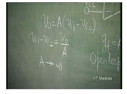
If A tends towards infinity, V i 1 minus V i 2 tends towards zero because A is coming in the denominator. V i is...or, V i 1 minus V i 2 becomes zero; or V i 1 becomes equal to V i 2. This error that sustains finite output is zero. That means, in this case, V naught should be finite. This is important. As long as V naught is finite, V i 1 is very nearly equal to V i 2 in all operational amplifier circuits.
