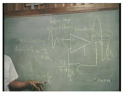
The biasing, etcetera, these are automatically taken care of. If you bias it plus V s and minus V s, the person in...who has designed this op amp has taken care that it is biased properly. The output is zero when the input is zero; no offset or very low offset.
