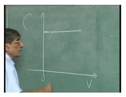
I am just drawing that to explain that. Now, when you apply negative voltage, it looks for plus charges. So, you get depleted layer there. The capacitance is capacitance of the oxide in series with capacitance of the depletion layer.
