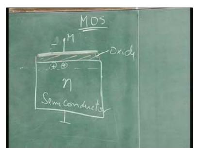
Depending upon the negative voltage that you apply, you get this. Till some maximum capability, the depletion layer reaches. Let me not get down into that. Now, what I say, if you take maximum value then the capacitance reaches a minimum at high frequency.
