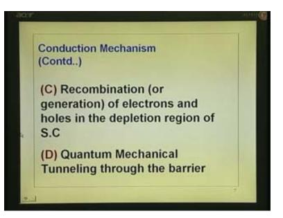
Recombination is in forward bias case generation in the reverse bias case of electrons and holes in the depletion layer. B and C what we have discussed just now, both are same ultimately, it is a forward bias case.
