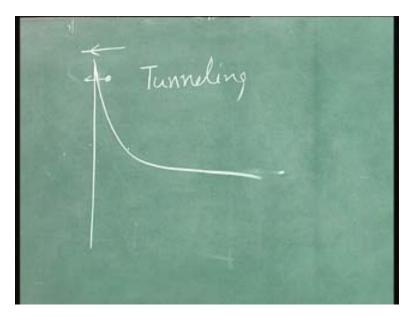
Barrier is wide here maybe 200 armstrongs, 300 armstrongs or even .1 micron but when you go to the top what we are talking of thermionic emission is the injection of electron across that barrier A. What we are talking of is the electrons which have energy here. They find that the barrier width is very small. That is quantum mechanical tunneling.
