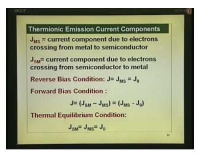
$J_{MS}$  the current component due to electrons crossing from the metal to semiconductor,  $J_{SM}$  is current component due to electrons crossing from the semiconductor to the metal. Reverse bias condition, total current is actually equal to go back reverse bias condition the whole thing will be pressed down, so none of these carriers will have energy to cross, we have discussed this earlier.
