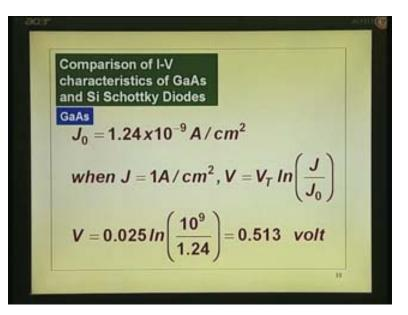
We have just now found out  $J_0$  is 10 to power minus 9 in gallium arsenide, silicon it is 10 to power minus 7, now  $J_0$  is this quantity. Supposing I say J equal to 1 ampere per centimeter square, corresponding voltage across the junction will be  $V_T$  long J by  $J_0$  where J is 1 ampere  $J_0$  is that quantity for gallium arsenide it is .513 volts, for silicon it will be, for silicon  $J_0$  is higher therefore V will be smaller .358.
