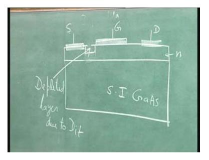
Now you will have ohmic contacts on two sides which will make n plus and metal. You will have a contact here like this. Notice I am putting it buried inside because you alloy it n plus into that and on that you have got the metal, so that is the source. Similarly, I have got drain here and this is the gate, this is the free surface that we are talking of.
