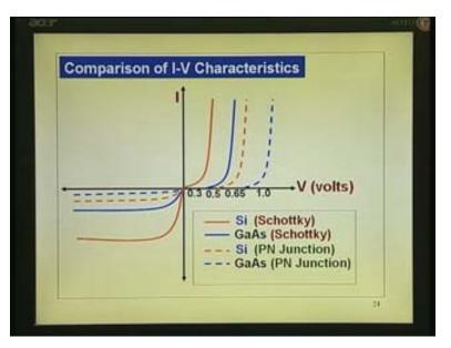
Schottky barrier blue that is gallium arsenide about .5 volts for a current of 1 ampere per centimeter square and silicon the forward voltage drop is smaller. Corresponding reverse currents I have shown here, gallium arsenide reverse current is smaller compared to silicon schottky, so these two, we will do the comparisons between the pn junction of gallium arsenide with metal semiconductor contact of gallium arsenide and pn junction of silicon metal semiconductor contact in silicon.
