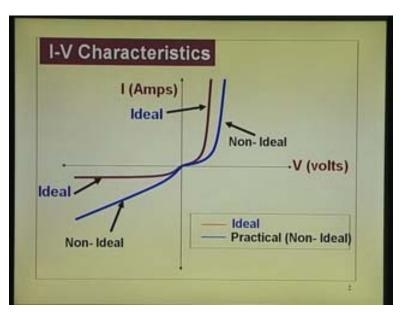
We have seen, or experiments have shown that the I-V characteristics deviate from the ideal characteristics. For example, the reverse current does not saturate, it will keep on increasing. Forward  $I_0$  e to power of, instead of V by Vt, it is V by nVt. That is less increases less rapidly with voltage.
