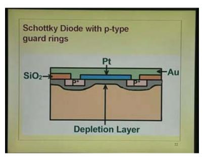
This is the p-type guard ring or p plus guard ring. You can see the plot here shows the metal here; this is the oxide; this is the metal put over top of that and schottky is only here. This is actually a schottky which is shorting and the junction is shorted out here
