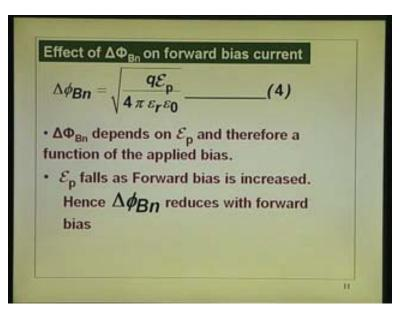
The delta  $phi_{Bn}$  is a value of phi at  $x_m$ , we have determined that is proportional to square root of peak electric field. Now before we go into that, we have derived this by taking the  $e_{external}$  is  $e_{peak}$  into x. Let us see whether it is valid at x equal to  $x_m$ . For that you must find out how much  $x_m$  is. Let me just give you some numbers their.
