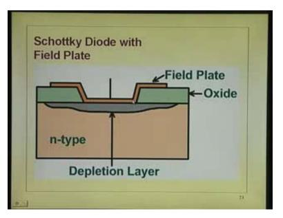
This in practice you need to make provision for reducing the field crowding, which would give rise to large current, particularly in the reverse direction due to quantum mechanical tunneling effect and image force lowering effect.
