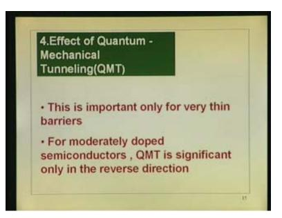
So now let us take one more phenomena because these two actually, the image force lowering effect and the quantum mechanical tunneling effect join hands together to spoil the reverse characteristics. Now if you recall what is this quantum mechanical tunneling? This is the fourth phenomena that we are discussing now, the causes for ideality.
