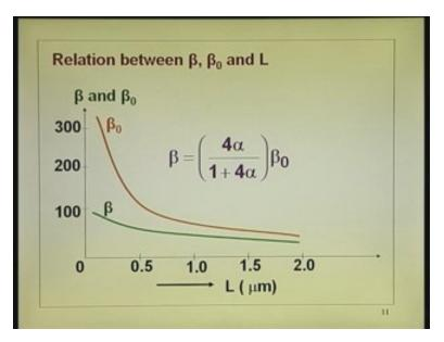
This is the factor. Finally, this term is what  $I_{DS}$  is and this is the factor which determines what transconductance is. Transconductance is delta  $I_{DS}$  by delta  $V_{GS}$ , which is nothing but twice beta into  $V_{GS}$  minus  $V_{threshold}$ . So you want beta to be high, if beta is high only your transconductance is good. What do we think usually from this expression is from long channel analysis what you think is, what is beta<sub>0</sub> even C<sub>s</sub> W by 2L.
