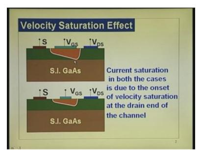
Current saturation is due to onset of velocity saturation in both cases at the drain end, the velocity saturation at the drain end. In long channel devices it coincides with the channel pinch off. This equation is not valid, it cannot be used really or determining  $V_{DS(sat)}$  in general case.
