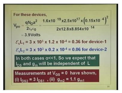
This is 3 times in the short channel device .2 microns channel device. This is almost constant. There is something wrong some where or some parameter is changing, so what it is actually we should have to analyze and see, in fact what parameter that getting affected will be the threshold voltage itself.
