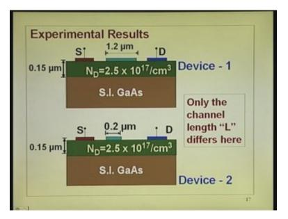
For this device the pinch off voltage for the doping and the thickness is to estimate substitute for q  $N_D$  2.5 into 10 to the power 17 and a is .15 into 10 to the power minus 4, thickness is .15 the channel thickness in this case and putting all these things it is 3.9 volts quite large pinch off voltage, so your doping is high.
