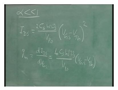
This is correct there is nothing wrong in that. What we can expect is  $I_{DS}$  should be now independent of channel length, whether alpha is .36 and .06; alpha is very much less than 1. Therefore you must get that and  $g_m$  also should be independent of channel length. But now what they observed when we made this experiment is, in both the cases alpha is less than 1. We expect that  $I_{DS}$  and  $g_m$  will be independent of channel length.
