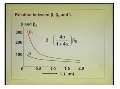
I illustrated the numbers, I have quickly gone through that but as this equation itself it tells that transconductance does not improve if you reduce the channel length, if you are in the region of short channel devices. Let us see that. Dream what happens? What we saw is this is the channel equation, beta<sub>0</sub> into 4 alpha by 1 plus 4 alpha, alpha very much less than 1 that is equal to 4 alpha the factor.
