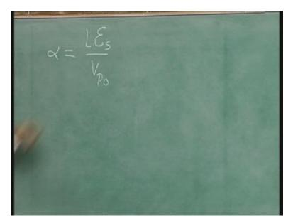
In general, what you do is, you approximate the velocity field characteristics, try piece wise linearization V is proportional to electric field, till the electric field is  $E_{s}$ , saturation field and up to that point V is equal to  $mu_n$  into E for E less than or equal to that. It is valid up to this point and beyond that point velocity is equal to saturation velocity. And saturation velocity is given also by this equation is valid try it up to that point.
