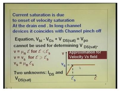
Now the two equations, I have just gone through it and quickly go through that, so for E less than E of s that is in this region that is from the source end close to the drain end of the channel, you can write that equation.
