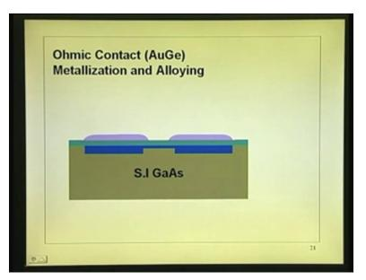
Make Ohmic contact, you want to form the gate contact finally without subjecting to any heat treatment. So make the Ohmic contact.
