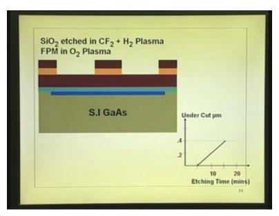
Then etch this particular layer silicon dioxide using a plasma of  $CF_2$  and  $H_2$  plasma we etch this. This particular top layer is acting as a mask for etching this one, it is protecting that. Now, this is photo resist; this is photo resist. Without this layer you cannot do the etching. So use this silicon dioxide as mask when you etch this one.
