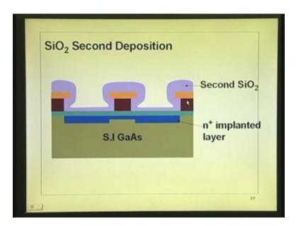
This n to the power plus implanted layer, now just notice what you do is deposit another layer of silicon dioxide; you can do that at low temperature, plasma deposition. 200 degree centigrade you can deposit using this silicon dioxide. That is how it comes. See, I deposit every where it is conformal deposition so it takes the shape of that. That is the oxide that we deposit. That is the second  $SiO_2$  layer.
