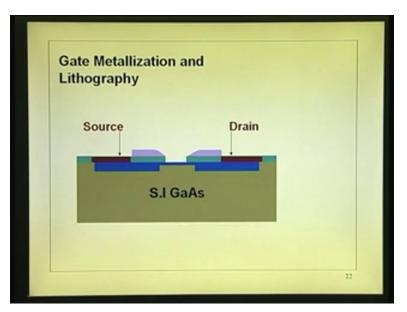
By lithography, you can precisely lift this portion because there is no oxide there. It is a very thin layer just about 1000 armstrong or less. So, you can etch it even a dip etching will do, but you can put photo resist remove that portion. Now you can see, you can do lift off technique again for realizing metal semiconductor contact only here.
