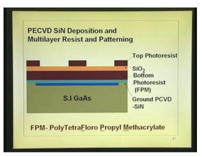
Another photo resist layer there, you can have bottom photo resist silicon dioxide then photo resist, flattering that, open the window there. Now, you can see you are getting an equivalent of that T gate portion now, the center. Etch top photo resist I already shown you masked, developed.
