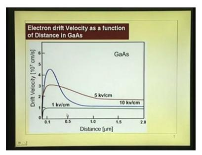
Now, let us take 10KV per centimeter you can see that goes to the peek, same peek value. But, x-axis distance because you multiply time into the velocity by about 0.5 microns, it has almost reached. In fact even write up to about 0.75 microns the velocity is much more than 10 to the power 7 per centimeter.
