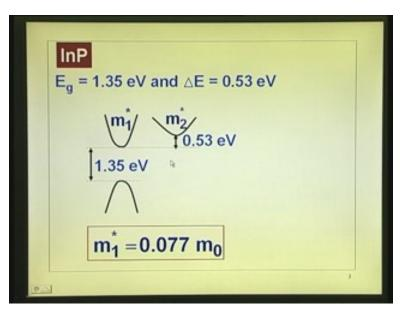
Also the other materials like indium phosphate, they have similar characteristics, because the energy band gap is 1.35 electron volts and this gap is 0.53. Now, this has some impact on the peek electric field and also the energy required transferring the electrons from here to here. They are more than that of gallium arsenide. Gallium arsenide required 0.36 electron volts. Now, this was more that means you could have higher fields.
