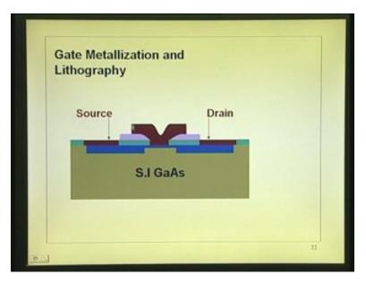
In the sense, put photo resist every where only in this portion so if I keep photo resist everywhere except this portion I put it in acetone, the photo resist from everywhere with the metal lifted off you will left to this.
