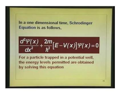
That is the famous Schrödinger's equation that we always see. We follow this particular equation. So psi is a probability wave function; psi square is the probability of finding the particle in a volume with certain k; m is the mass; Planck's constant h bar is h by 2pi, h is Planck's constant; E is energy of the particle as function of x and momentum. V(x) is the potential at that point.
