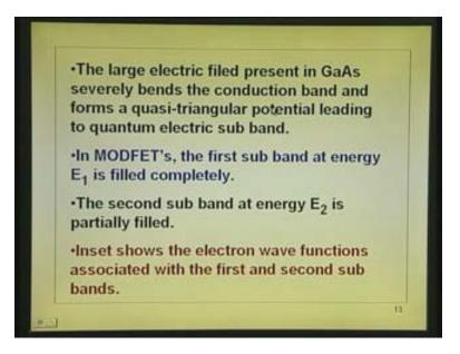
The large electric field present in the gallium arsenide severely bends and we have given more explanation on that band bending is more here, therefore, electrons are locked up there. In MODFET, we will go back to this afterwards, what we are telling is there are two levels there [are two energy levels in it] which I showed, let me just go into that.
