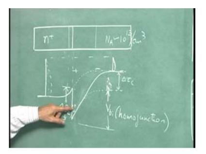
The potential phi of s here, the change built-in potential is there, E is actually larger than the built-in potential in the homo junction by an amount delta  $E_c$  by q.
