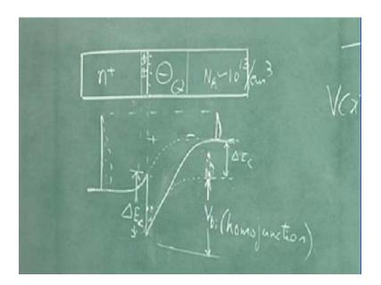
Whatever plus charge is present here that will be balanced by negative charge in the gallium arsenide and negative charge comes from where? Two regions are there: one this gap - notch mobile electrons; other one depleted layer; that is there are all these fixed charges and here there are fixed charges. So this is compensated by this charge and also these electrons there - that is the meaning of that.
