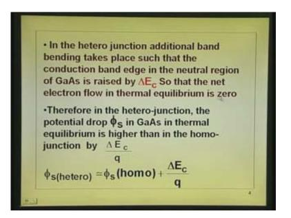
In the hetero junction additional band bending takes place such that conduction band edge in the neutral region of gallium arsenide is raised by delta  $E_c$ . So that, the net electron flow in thermal equilibrium is 0; whatever I have said now I have put in words here. Therefore, in the hetero junction, the potential phi of s in gallium arsenide, let us go back to this board and see.
