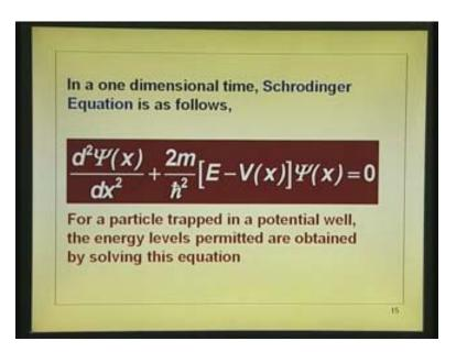
Let us see in couple of minutes we will just go through this quickly. For a particle trapped in a potential well, the energy levels are permitted to occupy that is what we are telling the moment there is a probability like this, there are discrete energy levels which the electron can take that is obtained by solving this equation.
