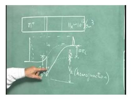
These electrons are located here in the undoped gallium arsenide region. They have been supplied from these dopents; all these electrons come from here, because, their donors are here (Refer Slide Time: 18:15 min). So, these electrons from here have fallen down here from a higher energy to that level; they remain there, because, it is like pouring water into
