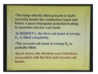
The second sub level energy  $E_2$  is partially filled. See after all if there are two levels one band will get filled completely, then only the next band will get filled up; that is the implication of that.
