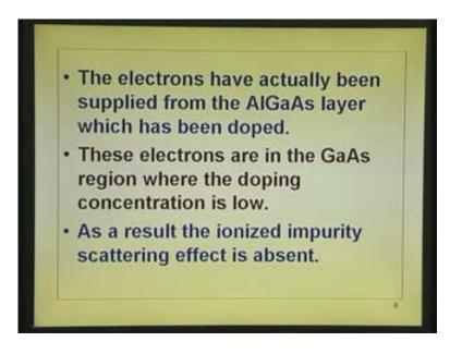
These electrons are gallium arsenide region where the concentration is low; what have we gained out of it? As a result ionized impurity scattering is virtually absent. As a result, this we have projected earlier as diagram.
