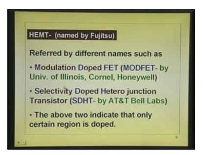
Now here the modulation doped means actually it is doped insulated regions. Your doping is modulated; how do you modulate? One layer undoped, another layer doped; that is all it is done. Then you call it up selectively doped hetero junction transistor by AT & T Bell labs and you do not have time to say selectively doped hetero junction transistor, you do not have time to say SDHT.
