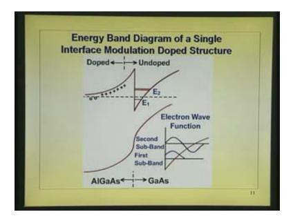
If there are two energy levels, the even levels will be filled first, completely. If you keep on dumping electrons into this notch by increasing this delta  $E_c$ , you will have electrons rising up to this level or by increasing the doping, you may have electrons going into this region. Initially the  $E_1$  level is filled up and it breaks up into a band instead of one level, that is what is put here. (Refer Slide Time: 47:39)
