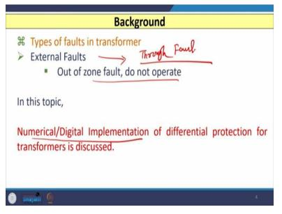
Sometimes in some cases they are also called as the through fault. So, whenever such type of fault occurs outside the range of the CT of the transformers connected on both sides of the winding of the transformer, then this relay should not operate in this case. So, we want stable operation of the relay in this situation. However, in this lecture we are going to concentrate more on digital or
