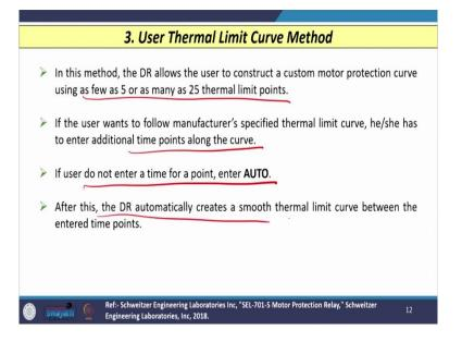
Now, let us see the third method that is nothing but the user thermal limit curve method. So in this method, the digital relay allows the user to construct the custom motor protection curve. So, whatever curve we want to construct based on whatever input we give you that is to be constructed. And that we can construct the curves as few as let us say 5 or as many as 25 thermal limit points we can have and based on that the relay can construct the custom motor protection curve.
