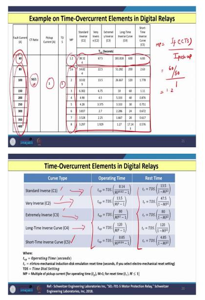
Now, with this background, let us see one example. So, here in this example, I have considered different value of fault currents in ampere starting from 60 to 400 A, I have considered CT ratio as 50 by 1, pick up current I have considered as 1 and TDS value is also I have considered or I have taken as 1. So, the first thing is I wish to calculate the value of MP. So, MP is nothing but my fault current refer to CT secondary / I pick up current.
