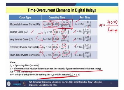
So, let us see if I wish to achieve this curve or this characteristic, then what are the different equations we can use in digital relays. So, if I use moderately inverse curve, then for that to calculate the time of operation of relay this equation is used  $t_{op} = TDS.\left(0.0226 + \frac{0.0104}{MP^{0.02}-1}\right)$
