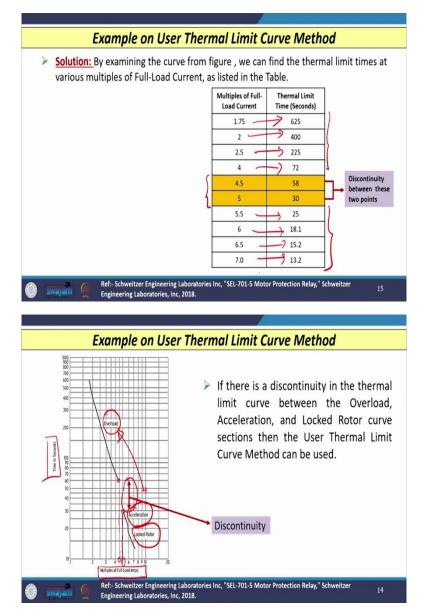
So, if we examine this curve, then we can find that the thermal limit times at various multiples of full load currents are listed in this table (as shown in above slide). So, what I have done, you
