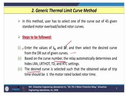
Now, let us discuss the second method that is known as generic thermal limit curve method. So, in this method user has to select one of the curve out of the several curves given by standard motor manufacturers or overload or locked rotor curves. So, most of the relay manufacturers they will provide several curves normally they provide let us say 40 45 or 50 curves.
