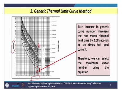
Now, let us see what are the different curves given or provided by the relay manufacturer. So, you can see here on the screen (as shown in above slide), the curve that is on x axis we have multiple of full load amps are given and on y axis the time in seconds are given and several curves are given. So, you can see that here several curves starting from here, 1 to 2 to let us say up to maybe 45, this curves are given here (as shown in above slide).
