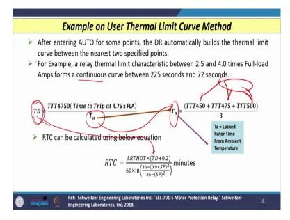
Now, after entering AUTO for some points, the digital relay will automatically builds the thermal limit curve between the two nearest points. For example, if a relay thermal limit characteristics that is between 2.5 to 4 times the full load amps from continuous curve between 225 second and 72 seconds, then the value of TD that can be calculated using equation,
