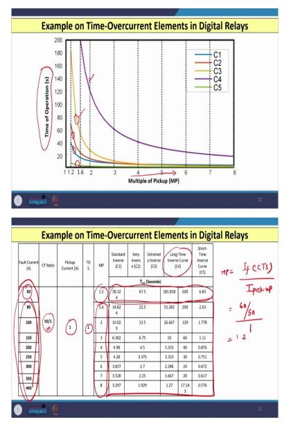
And if I plot the graph of this five curves, assuming on x axis I am taking multiple are pickup currents and on y axis I am taking time of operation in seconds, then you can see (as shown in above graph) that this are the characteristic of different curves starting from this is the characteristic of C4 curve. So, this C4 curve is nothing but your long time inverse curve.
