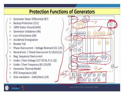
So, normally whatever 87G unit we used, where you have the three CT currents from terminal side and where we have the three CT currents here from the neutral side and that is compared both magnitude and phase wise, but if I go for turn to turn fault, then our conventional differential relay 87G unit is not capable to detect this turn to turn faults. The reason is the S differential relay works on the principle of Kirchhoff's current loss.
