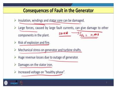
The point is if any fault occurs in the synchronous generator, then the consequences of this faults are the damage of the insulation or deterioration of the insulation windings can be damaged or core of the stator that can be damaged. So, this is one of the consequences of the occurrence of fault inside the generator if it is not cleared, sometimes large forces maybe because of the large magnitude of fault current that can also be there, which can damage the other components of the plant.
