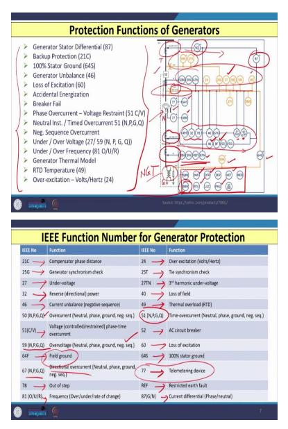
So, now, with this different device function number, if I look at the diagram of the generator (as shown in above slide), then you can see I have shown the diagram of the generator here. And you can see (as shown in above slide) that you have the generator available here and with this generator you have the generator field is also available here and this field you have the two important device that is 77 and 64F. So, you can see that here (as shown in above slide), you have the 77 number.
