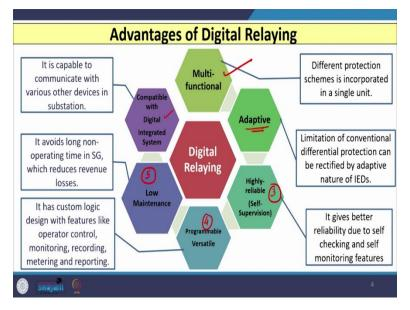
The reason for that is this digital or numerical or IED that is multifunctional in nature, so all types of functions or abnormalities that can be possible in a generator that is covered in a single unit. That is why digital or numerical relays are used. This numerical relays or digital relays are adaptive in nature.
