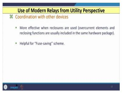
Further, we know that nowadays we are utilizing reclosers in the our conventional electrical system, and this is used just to improve the reliability of the system because if we reclose the system, we know that eighty to ninety percent faults are transient in nature, and they may die out after some time.
