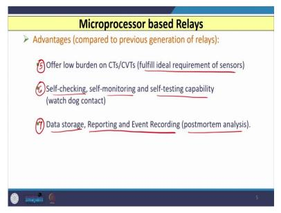
Then, we do have, the another advantage that is offered by this relay, that is the low burden imposed on the CTs, and CVTs. So, when we use microprocessor based relay, it imposes low burden on the CT, and PTs, or CVTs because of the lower VI requirement of the circuitry of this relay. And, this is going to fulfill the ideal requirement of any sensor, without utilizing the power of the acquired signal. It imposes low burden on the instrument transformers.
