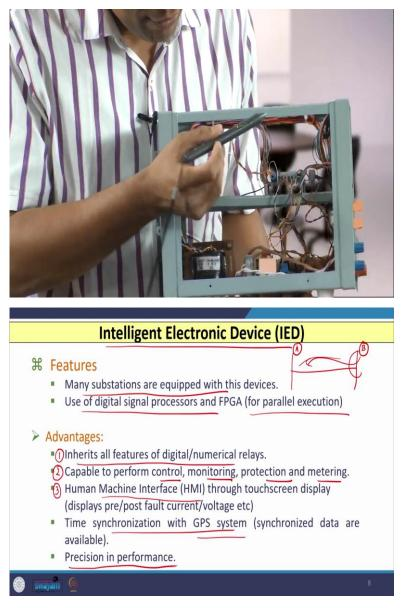
Whereas, if I consider the microprocessor based relays, then this relay looks like this. So, if you see, this is nothing but the microprocessor based relay, where you can see the processors that is available here, and below that some signal conditioning units are also available here. Now, if I consider the important advantage of this intelligent electronic devices, which are not available with microprocessor based relay, that advantage is, the time synchronisation with GPS.
