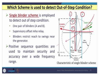
So, normally you can see here I have shown (as shown in above slide) the two vertical blue lines which is nothing but the pair of blinders and the supervisory offset, more related is used and the setting of this offset more relay is carried out in such a way that it will cover the generator XT'value. It will also cover the adjacent generator transformer impedance or reactance and some system reactance is also there and then these value of this delta that is observed.
