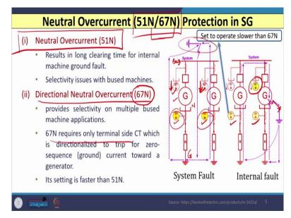
Now, the next category of protection we need for a synchronous generator that is known as the stator ground fault protection. So, for that let us consider the winding of one phase. So, this is the neutral side and this is the terminal side of the winding. And the one of the way to protect or to provide the protection in synchronous generator against ground fault in stator that is the use of over voltage relay.
