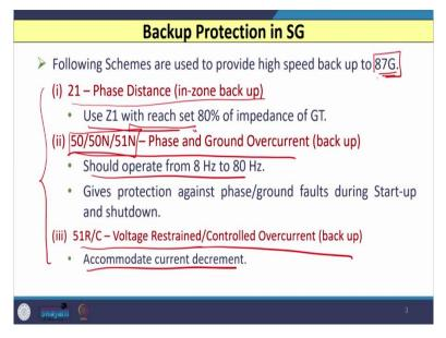
Now, in this class, let us discuss that what happens if my conventional 87G or differential relay fails to operate due to some reasons. We know that whenever faults are going to occur in the synchronous generator particularly in the stator of the generator, then the magnitude of current is very large. As I told you the normal case 210 Megawatt generator, the full load current is of the order of 10,000 ampere.
