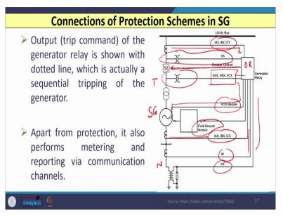
Now, using all these schemes if I summarize then let us see what different types of connections we need to give in the synchronous generator. So, here you can see (as shown in above slide) this is my synchronous generator and this is the neutral on the side of the synchronous generator and this is the terminal side of the synchronous generator and this is my digital relay for generator protection.
