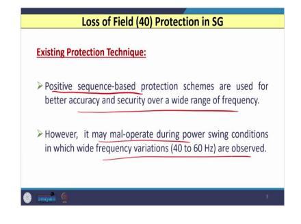
So, to detect to avoid this we need to detect the loss of field which is going to occur in the synchronous generator and for that the existing scheme that is going to use the concept based on positive sequence component. So, this scheme though they provide better accuracy and security for a wider range of frequency. But they may mal operate in case of power swing condition in which the frequency may vary from 40 to 60 Hz. So, this scheme may fail in that case.
