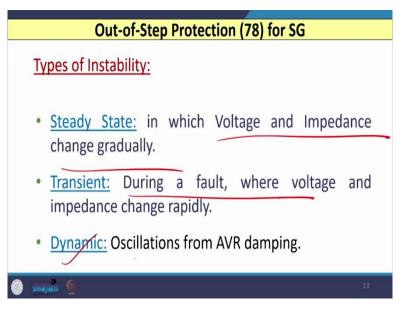
So, in this case that three types of instability are very important one is the steady state instability in which voltage and impedance change gradually. In case of transient instability, this is normally during a fault where voltage and impedances change rapidly and the dynamic instability is also there, where we will observe the oscillation from automatic voltage regulator damping.
