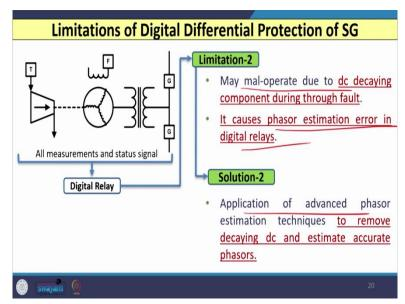
The second limitation of digital relay is this type of relay may mal operate in case of DC decaying component particularly in case of true fault or external fault. And in this case when such type of situation exists phasor estimation error is there in the digital relays.
