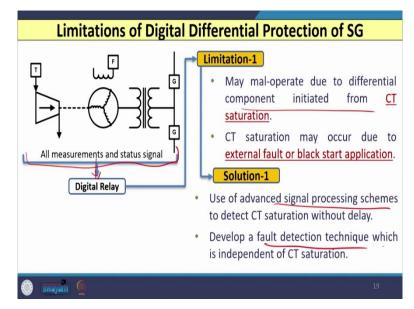
However, with this background let us see what are the limitations of digital differential protection of synchronous generator. So, you can see (as shown in above slide) that this is my generator with the prime mover and the associated generator transformer unit and we are acquiring the measurements and that is given to the digital relay. However, in most of the digital relay they may mal operate because of the CT saturation condition.
