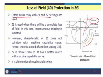
So, to achieve this normally in to detect the loss of field in synchronous generator the two types of relay settings are used. And normally they use the offset more relay with two settings Z1 and Z2. So, you can see (as shown in above slide) this dotted circle is Z1 setting and the full dark circle is the Z2 setting. So, here the Z1 setting is used when there is a complete loss of field.
