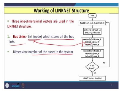
Once you have these two parameters end A and end B, you need to calculate three onedimensional vectors and these vectors are shown here as next, list and far. So, this next, list and far are the three one-dimensional vectors, which you need to calculate in LINKNET structure particularly, when you are dealing with algorithm 1 of the LINKNET structure. So, let us see what is the significance of these three one-dimensional vectors.
