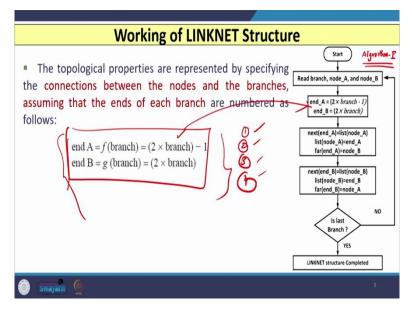
Now, when we consider this algorithm 1, this is my algorithm 1 (as shown in above slide). So, when I consider this algorithm 1, the topological properties that in this algorithm are represented by specifying the connection between the nodes and the branches. So whatever connection you are going to do between the node that is bus and the branches, because we know that a particular branch is connected between two nodes or two bus.
