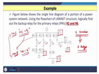
So, with this background, we will discuss one example. And in this example, I will just give you the highlights of this example. So, you can see (as shown in above slide) that here, the figure below shows the single line diagram of a portion of power system network. So here, you can see that four branches are there, this is my branch number 1, branch number 2, branch number 3 and branch number 4, four branches are there.
