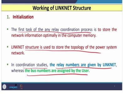
So, with this background, let us see how the LINKNET structure works. So, the first task of any relay coordination process is to store the network information optimally in computer memory. So, LINKNET structure is used to store the topology of a particular distribution network such that we can store that values optimally in the computer.
