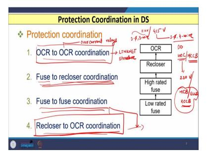
So, till now, what we have discussed is, that coordination of protection, in terms of four different aspects. The first is the coordination between two relays. So, OCR-to-OCR coordination, where OCR indicates the Overcurrent Relay. So, we have the coordination between overcurrent relays, that is one relay and the other relay.
