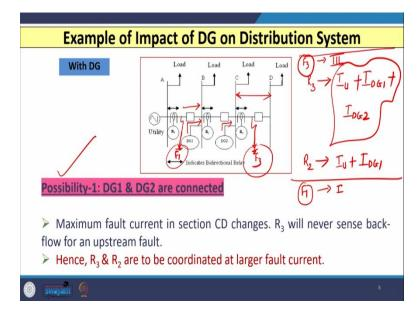
Now, let us consider same radial network but we have connected or we have incorporated distributed generators or distributed energy resources, maybe in terms of solar, wind and so on at different buses. So, when we connect the DG, let us consider different possibilities, so, first possibilities I am taking that 2 DGs, DG1 and DG2, are connected at bus B and bus C respectively, as shown in the figure.
