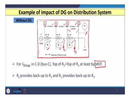
So, let us understand this thing. How the relay mis-coordinate, when we incorporate distributed generators in a radial distribution network with some example. So, here let us consider this system (as shown in above slide), in which the three sections are shown, section 1, section 2 and section 3. And these three feeders are connected between the four buses, bus A, bus B bus C and bus D.
