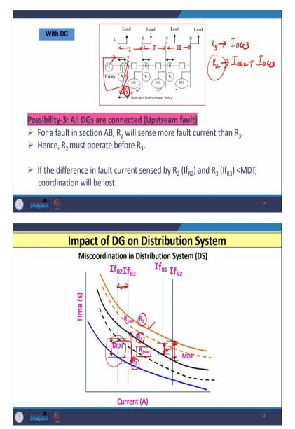
Now, let us consider the third possibility, where all the DGs are connected that is DG1, DG2 and DG3 are connected at bus B, C and D and the fault we are considering that is the upstream fault means those faults which are going to occur near the source. So, let us say, we have this is our section 1, this is our section 2 and let us say this is our section 3 (as shown in above slide). And fault that is going to occur let us say, at  $F_1$  in section 1. So, this is nothing but the upstream fault.
