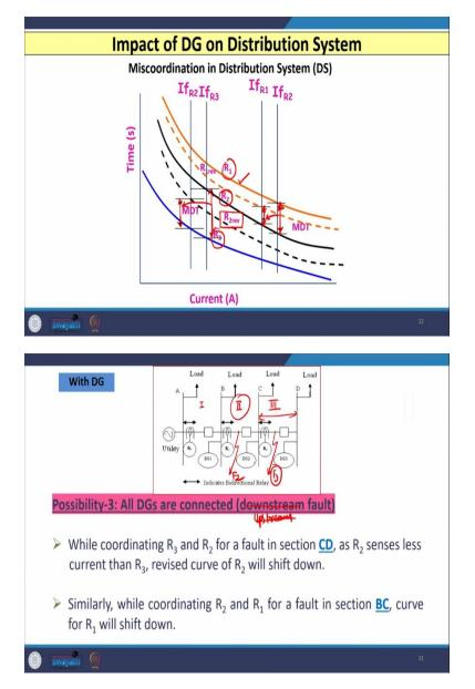
So, the  $R_2$  curve has to shift down, and you can see (as shown in above slide) that I have shown the characteristic of  $R_1$  with this color,  $R_2$  with black color and  $R_3$  with this original blue color. Now, the characteristic of  $R_2$  has to shift below. So, you can see I have mentioned here I  $R_2$  revised. So, which is shown by dotted black color. So, now, you can see in earlier case between  $R_2$  and  $R_3$ , this much margin is available (as shown in above slide).
