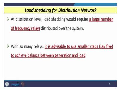
Now, when we talk about the load shedding for distribution network, then at distribution level load shedding would require large number of frequency relays. So, with so many large number of frequency relays, it is advisable to use smaller steps, let us say three steps or five steps to achieve the perfect balance between the generation and the load.
