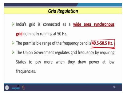
Now, the important aspect is the grid regulation. So, we know that our Indian grid or network is connected to a wide area synchronous grid which is normally running at 50 Hz. In other countries the fundamental or base frequency is 60 Hz. The permissible range of frequency for 50 Hz fundamental frequency is 49.5 Hz to 50.5 Hz.
