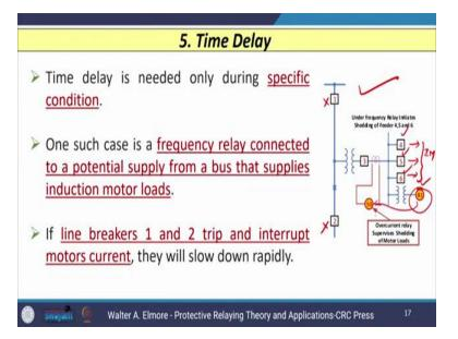
However, this long-time delay of 30 cycles that is not consistent or that is not in coordination with the load shedding requirement or load shedding requirement of the scheme. Hence, if we wish to achieve more effective method then the only option is we have to supervise this under frequency relay by overcurrent relay. So, that is why this 81 relay is all supervised with the overcurrent relay 50.
