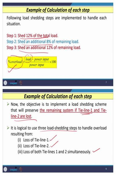
Now, when we design the load shedding scheme, then as we have seen that we will go for the three load shedding steps. So, these steps should be implemented in the following situations. So, in step 1, we have to shed 12 percent of the total load. In step 2, we have to shed the additional 8 percent of the remaining load.
