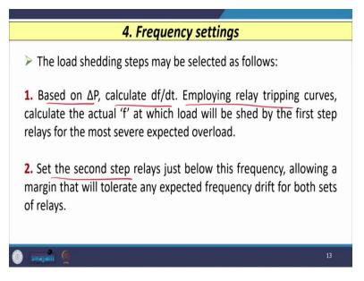
So, for frequency settings load shedding steps may be selected as follows and there are five steps which we need to follow. So, in step number 1, based on the  $\Delta P$  change in active power, we have to calculate the rate of change of frequency. Once we have the df / dt, then employing the relay tripping curves, we have to calculate the actual value of frequency at which the load will be shed by the first step relays for the severe most expected overload condition.
