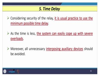
Now, the fifth factor which is going to affect the design of an intelligent load shedding technique, that is the time delay. So, it is the usual practice to use the minimum possible time delay. When the time is less the system can easily cope up with severe overloads and all necessary interposing auxiliary devices that should be avoided, so that we can have this. But however, one important condition is that time delay is needed only during specific situation.
