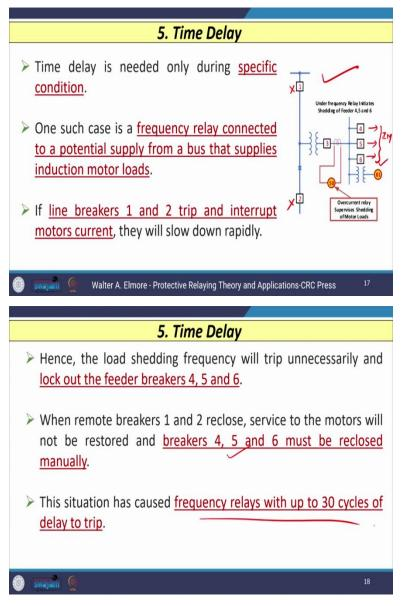
For example, one such situation we can consider using this diagram, where the frequency relay is connected. So, you can see that 81 is my frequency relay which is connected on the secondary of
