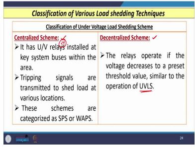
Now, let us see what are the classification of various load shedding techniques. So, the first type of classification of the load shedding technique that is one is centralized scheme and other one is the decentralized schemes. So, centralized scheme has under voltage relay that is 27 relay is there that is installed at key buses within the area or network. And tripping commands are initiated or transmitted to shed the load at various locations.
