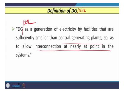
So, let us first discuss how we define the distributed generator or distributed energy resources. So, DG or distributed energy resources is defined as a generation of electricity by facilities that are sufficiently smaller than central generating plants so as to allow interconnection at nearly point in the system. And this point, where you are going to connect the generators, either grid that is known as point of common coupling PCC.
