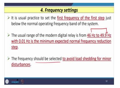
Now, it is usual practice to set the first frequency of the first step just below the normal operating frequency band of the system. The usual range of the most of the digital relays that would be from 46 Hz to 49.9 Hz with 0.01 Hz is the minimum expected normal frequency reduction step, assuming 50 Hz is the fundamental frequency.
