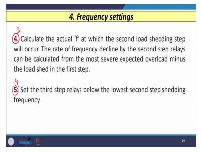
In the third step, we have to calculate the actual frequency at which the second load shedding step will occur. So, the rate of frequency declined by the second step of relays that can be easily calculated from the most severe expected overload minus the load shed during the first step. And then in the fourth step, we have to set this third step of relays below the lowest second step shedding frequency.
