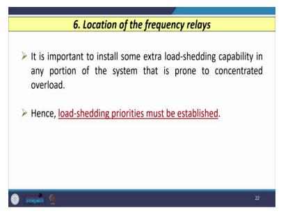
So, it is important to install some additional or extra load shedding capability in any portion of the system that is prone to the concentrated overload. Hence, load shedding priorities that need to be established when we design intelligent load shedding scheme.
