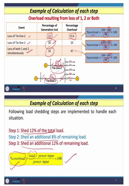
So, if I use this each and every case, let us say in case 1, there is a loss of tie-line-2. So, when there is a loss of tie-line-2 that is in this figure, this is not there, because of some reason, this breaker and this breaker both will become open. So, then there is a loss of tie-line-2. And this tie-line-2 is carrying the percentage of the load that is 12 percent. So, the generation lost that is 12 percent.
