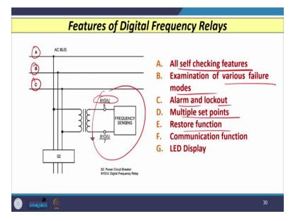
Now, with this let us see what are the features of digital frequency relays? So, here you can see (as shown in above slide) I have shown the three conductors A, B, C. And when you have the frequency relay, as I told you, it comes with 81 number and you have 81 over frequency unit. So, you have the frequency sensing that is to be carried out from the secondary of PT and digital frequency relay which is used by most of the utilities all have all self-checking features.
