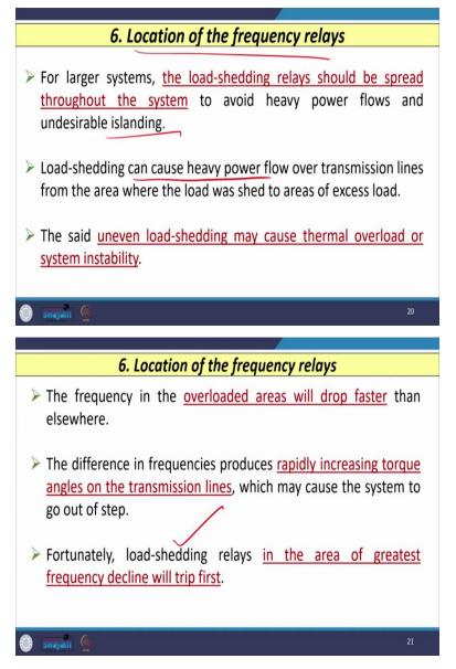
Now, the next step, which we need to consider for the design of intelligent loads shedding scheme that is the location of frequency relays. We know that for larger networks load shedding relays should be spread throughout the system to avoid heavy power flows and undesirable islanding condition, what is islanding condition? That we will discuss later on. The load shedding can cause heavy power flow over the transmission lines from the area where the load was shared to the areas of excess load.
