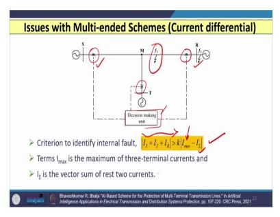
Now, let us see the second category of scheme multi ended schemes. So, the best example is the current differential. So, here (as shown in above slide) I have shown the three terminal line with a differential relay unit which is going to take the currents from the substation S substation R and substation T and all the three currents are available here.
