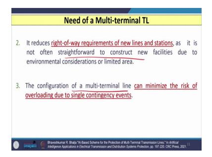
The second is if I have multi terminal or three terminal line, it reduces the right of way requirements for new lines and stations as it is not often straightforward to construct new facilities due to environmental considerations or limited area. So, it is not possible to construct a new transmission line which is very difficult, because of the three reasons which I have mentioned earlier. So, the only option is the multi terminal line or three terminal line.
