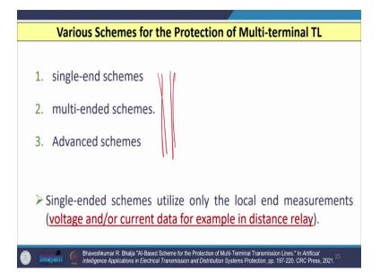
So, let us see what are the various schemes that is used for the protection of multi terminal transmission lines. So, normally the people use the three schemes for the protection of multi terminal transmission lines. The first one is the single end schemes as the name suggests, it will take only measurement from sending end or local end. The second is the multi ended schemes can take the measurements from several buses.
