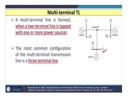
Now, let us consider what is multi terminal or three terminal transmission line? So, a multi terminal line is formed, whenever a two terminal transmission line is tapped or for when we take the tapping from the two terminal transmission line with one or more power sources, let us say we have a tapping tap point M and we have taken one tap and that is connected with source T at substation T. So that is known as multi terminal line.
