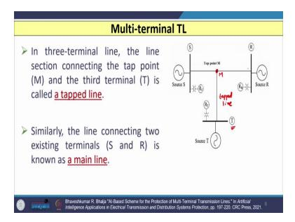
Now, if I consider the three-terminal transmission line, then the line section connecting to the tap point we have a tap point that is M to the third terminal that is substation T that is known as the tap line. So, this is known as the tapped line, because we have taken tappings from the conventional two terminal line. Similarly, the other two sections that is connected between S and M and between M and R this R is nothing but our main line.
