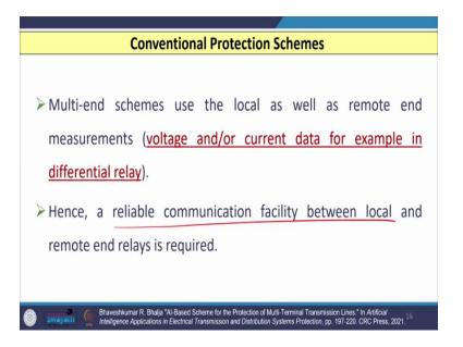
Multi ended schemes, that uses measurements from remote as well as some other buses. So, voltage or maybe current or maybe both the quantities. Then let us say example is differential relay is the best example used for transmission line. Hence, a reliable communication facility between local and remote end is required if you use multi ended schemes, because you need a measurement from the remote or maybe several other remote buses also.
