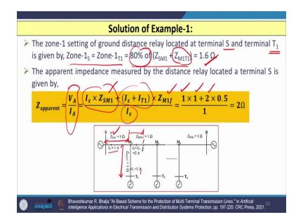
So, the zone 1 setting if I just calculate for the relay located at terminal S and terminal T<sub>1</sub>, then that is nothing but the Zone-1<sub>S</sub> = Zone-1<sub>T1</sub> = 80% of  $(Z_{SM1} + Z_{M1T1}) = 1.6 \Omega$ .
