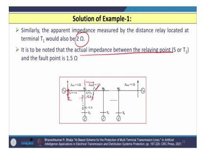
Similarly, you can calculate the apparent impedance measured by the distance relay located at
