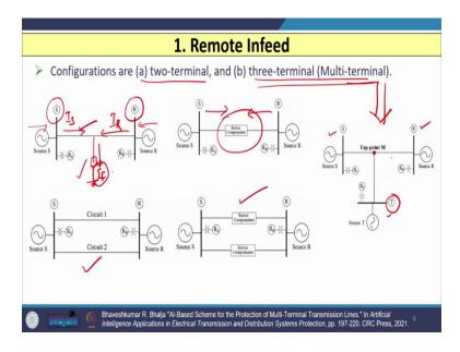
So, let us see what is remote infeed? So, when I consider the remote infeed situation or condition, we have to consider the two configurations of the transmission lines, the first configuration is the two terminal transmission lines. So, two terminal means we have the transmission lines connected from both the buses that is sending end, receiving end. So, we have the source at the receiving end as well as we have the source at sending end.
