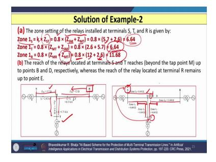
So, if I calculate the first part that is the zone settings of the relay located at S, T and R, then the relay located at S that is nothing but the k times the  $Z_{ST}$ . So, here you can see K is my 80 percent is the I am assuming that the reach of first zone is 80 percent so k is 0.8.
