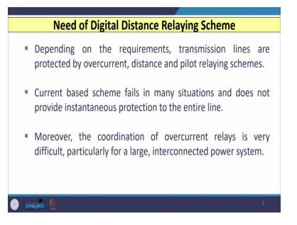
Now, let us see what is the need of digital distance relaying scheme? So, we know that depending upon the requirements, transmission lines are usually protected by either overcurrent relays, distance relays or pilot relays. Current base relays or the protection based on the overcurrent relays, that fails in many situations and that overcurrent relay does not provide instantaneous operation throughout the entire length.
