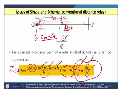
Now, if I consider what is the apparent impedance seen by the relay installed at terminal S, then it can be given by the measured value of impedance by relay, let us say at substation S or terminal S that is nothing but the voltage drop between S and M.
