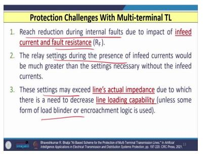
Let us see what are those challenges? The first challenge is the reduction in reach in case of internal fault because of the impact of remote infeed and fault resistance  $R_F$ . The second is the relay settings during the presence of infeed current that would be much greater than the settings which is required
