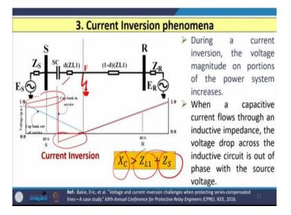
The third issue is the current inversion phenomena. So, during a current inversion the voltage magnitude on portion of the power system increases. So, you can see in earlier case when voltage inversion is there both the voltages whether the capacitor bank is there or not it reduces whereas, in the current inversion when capacitor bank is not connected, the voltage is shown by this blue line at each and every point throughout the line.
