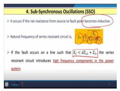
The fourth phenomena is known as sub-synchronous oscillations. So, this type of phenomena occurs when the net reactance from the source to the fault point that becomes the inductive So,
