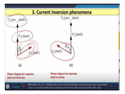
And if I draw the phasor diagram, then in that case when capacitor bank is out of service, you can see that the pre fault voltage and  $V_s$  both are in phase and your current is somewhere here and the theta line is here, but when the capacitor bank is available or connected in the line, then this Is reverses, because of these the apparent impedance seen by the relay that is again negative and hence the relay may not operate properly.
