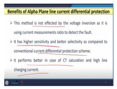
So, there are certain benefits of the alpha plane line current differential protection scheme. The reason is this method is not affected by the voltage inversion phenomena because it works on
