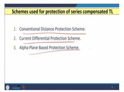
Now, to avoid this for all the four phenomenas that is the current voltage inversion, the nonlinearity introduced because of MOV and XC series capacitor and the last one that is the subsynchronous oscillations which are introduced because when XC value is greater than the dZL1 plus ZS. To avoid that normally three types of schemes are used one is the conventional digital distance relaying scheme, another is the differential scheme and another is the alpha plane scheme. (Refer Time Slide: 30:25)
