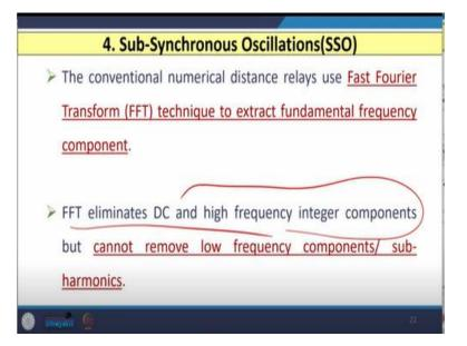
So, because of that whatever is the apparent impedance seen by the relay that is also oscillating in nature. So, in this case, the conventional numerical distance relays normally use fast Fourier transform techniques to extract the fundamental frequency components. So, this is basically phasor estimation techniques though FFT eliminates decaying DC component and high frequency integer components, but this is not capable to remove low frequency component or sub-harmonics.
