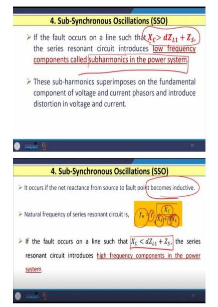
On the other hand, if the reverse is the case that means, when, here high frequency components are introduced when  $\frac{\text{XC}}{\text{XC}}$  is less than this dZL1 plus ZS, but is reverse is the case when  $\frac{\text{XC}}{\text{XC}}$  is greater than dZL1 plus ZS then this are going to introduce a low frequency component in the
