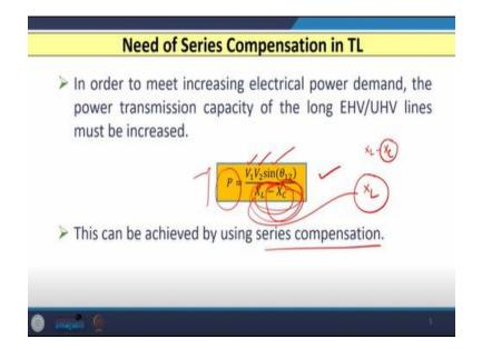
Now, let us discuss the second problem faced by digital distance relay that is the series compensation. So, we know that in order to meet the increasing electrical power demand, the power transmission capacity of long transmission line needs to be increased and this power to be transmitted by any transmission line that is governed by this equation.
