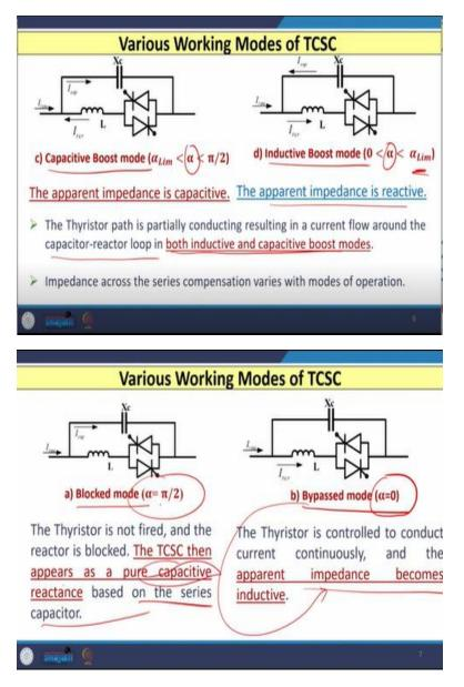
The third mode in which the TCSC module can work that is the capacity boost mode, where the value of alpha varies from alpha limit to the pi by 2 and the apparent impedance in this case is capacity and the fourth mode is the inductive boost mode, where the alpha varies between 0 and alpha limit and here the apparent impedance is reactive in nature.
