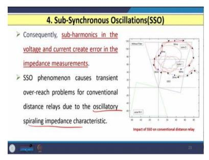
So, because of that the sub-harmonics in the voltage and current create the error in the impedance measurement. So, particularly you can see that in this case the impedance seen by the relay that is
