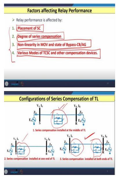
Now, when we consider the distance relay which is used for the protection of series compensated transmission line, then the performance of this relay is affected by several factors. The first factor is the placement of series capacitor as I told you, whether we are putting this at the middle or we are putting at the sending end only or we are putting at both end sending and receiving end
