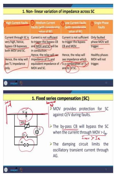
So, to understand that, let us consider four different conditions. The first condition is when the value of fault current is very high, let us say the three phase voltage short circuit occurs symmetrical fault occurs in that case, what would be the apparent impedance seen by the distance relay. So, when the magnitude of fault current is very high current through the series capacitor is very high and hence bypass circuit breaker bypass it both MOV as well as the series capacitor.
