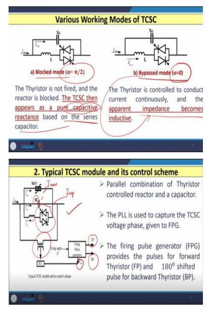
Now, there are four working modes of this typical TCSC module. So, let us see what are these four modes in which this TCSC can work? So, the first mode of this TCSC module is the blocking mode. So, in this mode, the value of alpha that is the alpha which is available here, that value of alpha is 90 degree or pi by 2. So the thyristor is not fired in this case when TCSC is working in
