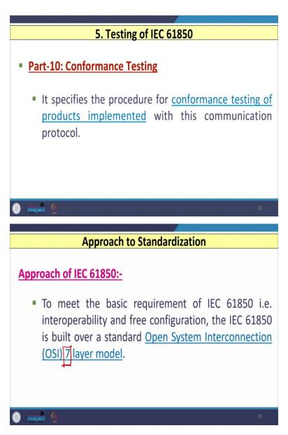
In part 10, the issues related to the testing of IEC 61850 that is mentioned, so part 10 conformance testing related information is given and in this it is specified that the procedure for conformance testing of product which we wish to implement with this communication protocol that is how it is implemented, so complete information related to this that is to be elaborated in this part 5 that is related to the testing of the IEC 61850.
