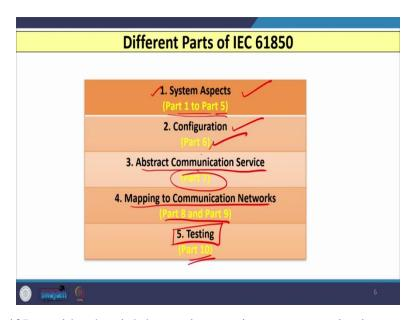
In the same thing if I consider the eighth part, in mapping to communication networks then in part 8-1 mapping to MMS and ISO oblique IEC for 8802-3 that is mentioned, in 80-1 guidelines are given in details regarding the exchange of information from a CDC based data model using IEC 60870-5-101/104. In ninth part that is the 9-2, sampled values, how we can have the sampled values over ISO or IEC 8802-3 that is mentioned.
