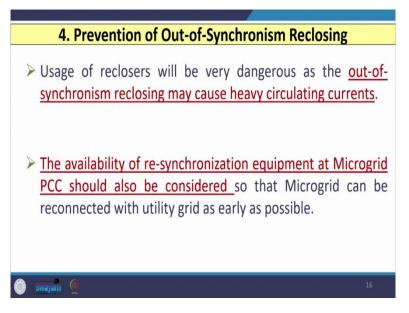
So, if we reclose this thing, then large circulating current fuel flows and that is going to damage the loads which we have connected in the distribution network or in the microgrid. So, availability of resynchronization equipment at microgrid PCC should be always considered. So, microgrid can be reconnected with utility as early as possible. (Refer Slide Time: 13:25)
