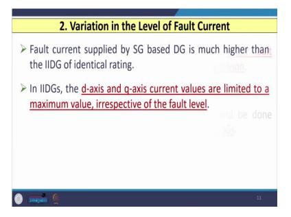
Now let us see the second issue variation in the level of fault current. So, we know that fault current supplied by the synchronous generator base distributed generator is much higher than the inverter interface distributed generators of the same rating. So, in case of inverter interface distributor generators, the d axis and q axis current values are limited to a maximum value irrespective of the fault level.
