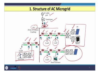
So, here the utility grid is there through the transformer, we have a bus which is known as point of common coupling. So, before point of common coupling, we have a relay along with the circuit breaker So, that if we wish to disconnect or isolate this utility grid from the rest of the system that we can do by opening this circuit breaker. Then we have feeder on which several lines are connected like we have line 1, line 2 and line 3, line 4, line 5, line 6, line 7 and line 8.
