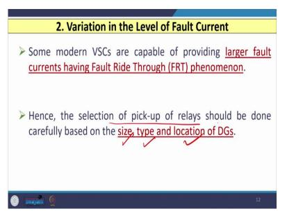
Some modern voltage source converters are capable of providing larger fault current having fault right through phenomena. Hence, when we select or decide pick up of the relays then we have to decide this very carefully based on the size, type and location of the distributed generators or distributed energy resources.
