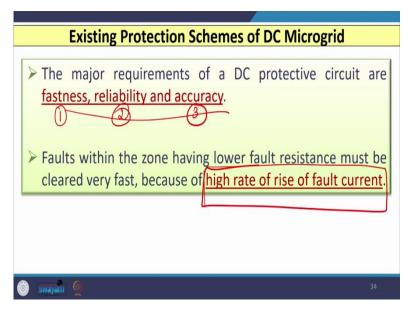
So, we can say that the major requirements for any DC microgrid if I consider protection wise then the protective scheme used for DC microgrid, it has 3 important characteristic that is one is the fastness, second is the reliability and third is the accuracy. So, faults within the zone having lower fault resistance must be cleared very fast, because of high rate of rise of fault current. So, this type of fault that should be cleared instantaneously.
