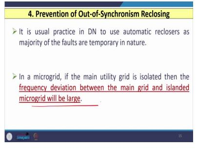
The fourth is the prevention of out of synchronism reclosing. Now, we know that it is usual practice in distribution network to use auto reclosers as majority of faults are temporary in nature 80 to 90 percent faults in distribution networks, they are temporary or transient in nature and they die out maybe after one cycle or one and a half cycle.
