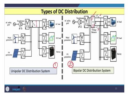
Now, let us see what are the types of DC distribution. So, there are 2 types of DC distribution. The first is the unipolar DC distribution system and second is the bipolar DC distribution system. The difference is here you can see that in unipolar DC distribution system only one voltage level is there.
