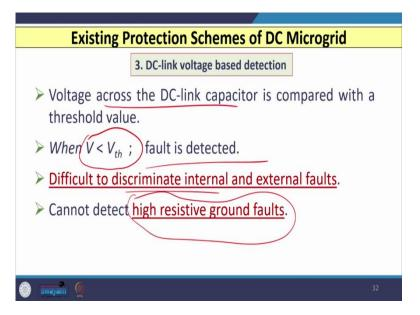
So, the third type of scheme that is DC link voltage-based detection scheme, in this scheme voltage across the DC link capacitor is compared with some threshold value. So, when V is less than V<sup>th</sup> then the fault is detected otherwise it is some external condition or normal condition. However, it is difficult to discriminate between internal and external fault using this scheme and this scheme also faces difficulty in detecting high resistive ground faults.
