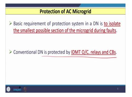
Now, let us see protection aspect of AC microgrid. So, the basic requirement of any protection system if we are using for distribution network is to isolate the smallest possible section of the microgrid during faulty situation. So, conventional distribution network is protected by inverse definite minimum time overcurrent relays associated with circuit breakers.
