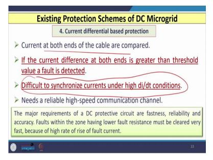
So, the fourth type of scheme that is known as current differential base protection scheme. So, in this scheme current at both ends of the cable are compared. So, you need remote as well as the local end data if the current difference at both ends is greater than the threshold value, then
