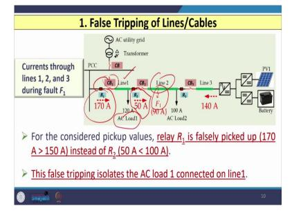
Now, let us say fault is going to occur on line 2 at  $F_1$  with a current 90 A. So, there is a redistribution of current and now you can see through relay  $R_1$  170 A current flows and through relay  $R_2$  50 A current flows, the pickup setting of relay  $R_1$  is 150 A. So, as 170 A is greater than 150 A. So,  $R_1$  will picks up and it will initiate the command and your circuit breaker 1 that is going to isolate in this condition.
