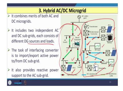
Now, let us see the third type of microgrid that is hybrid AC DC microgrid. So, hybrid AC DC microgrid is a combination of both AC microgrid and DC microgrid. So, you can see that this is the structure of hybrid AC DC microgrid and you can see there both AC and DC are shown here. So, you can see that this the scheme with the green color that I have shown here, these are your AC microgrid and all this blue color they are the DC microgrid systems.
