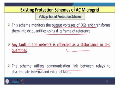
The third type of scheme that is known as voltage-based protection scheme. So, this scheme monitors the output voltage of the distributor generators and then transforms the face quantities
