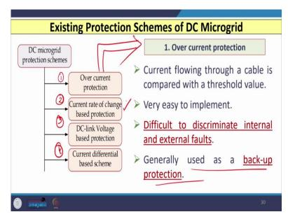
Now, let us see what are the existing protection schemes for DC microgrid. So, for DC microgrid 4 types of schemes are used and that is the overcurrent. So, first is the overcurrent protection scheme. So, the current flowing through a cable that is compared with some threshold or pickup or pluck setting, So, it is very easy to implement this scheme.
