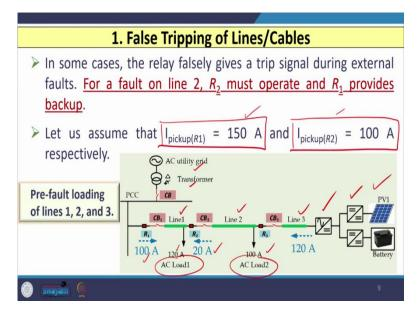
So, to understand this phenomenon, let us consider a network in which utility grid is there, which is connected at PCC through transformer and we have a line 1 line 2 and line 3 are connected with several loads AC load 1 and AC load 2 and on the right-hand side we have a PV based generator with battery which suitable converters are there that is DC to DC and DC to AC converters are there.
