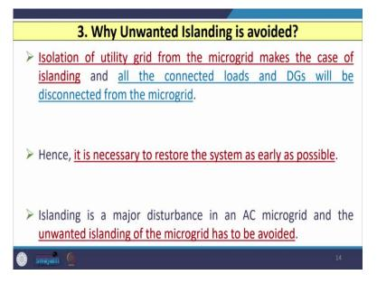
Now, isolation of utility grid from the microgrid that makes the case of islanding and all the connected loads and DGs will be disconnected from the microgrid. Hence, it is necessary to restore the system as early as possible. So, islanding is a major disturbance for AC microgrids and unwanted islanding that should be avoided as far as possible.
