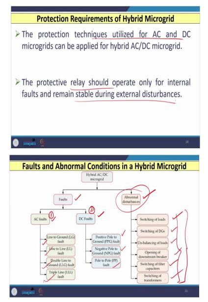
So, protection requirements of hybrid AC DC microgrid if we consider than protection techniques utilized for AC and DC microgrids can be applied to hybrid AC DC microgrid. The protective relay should operate only for internal faults and remain stable for any external disturbances as we have discussed earlier. So, any of this disturbance relay should not operate.
