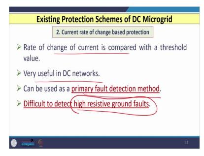
So, the second type of scheme is the current rate of change-based scheme. So, this scheme is based on rate of change of current and that value is compared with some threshold value. So, this type of scheme is very useful for DC network and it can be used as a primary fault detection method. However, it is very difficult to detect high resistive ground faults if I use rate of change of base protection scheme.
