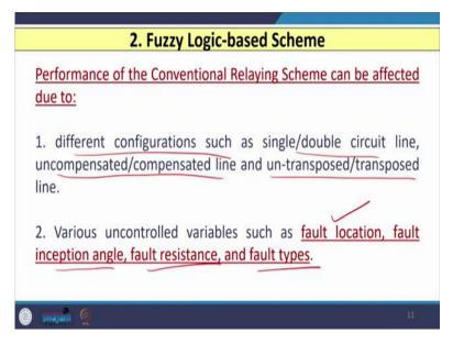
So, we know that performance of conventional relaying scheme that can be affected because of several parameters. For example, we have different configurations such as single or double circuit transmission line, we have uncompensated or compensated transmission lines, maybe series compensated and compensated and so on. We have un-transposed or transposed line.
