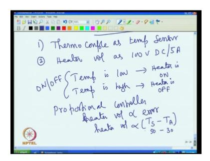
So, today's topic will be proportional temperature controller (No Audio From: 00:50 to 01:02). So, we use thermocouple as a temperature sensor (No Audio From: 01:07 to 01:16). Now, in this case we take second point is the heater voltage because heater voltage as 100 volt is required; we will see for various heater voltage how to design. But first we take heater requires assume 100 volt d c and then it needs assumes say 5 ampere
