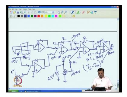
So, all that now comes is that I will get here; if the temperature difference is 50, suppose if this is 100. If the actual temperature is suppose, if a set temperature is the set temperature is 100 and actual temperature is 50; then I will get plus 50 millivolt here. So, here you will get error 50 millivolt for example here. So, this point gives me error voltage; so this voltage is nothing but T set minus T actual. Every one milli one degree
