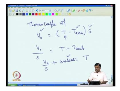
So, what is normally done is the measure the thermocouple voltage; thermocouple voltage is actually nothing but T minus T ambient into S. So, that is voltage, so voltage output. So, we know voltage output here and we know ambient temperature, we know
