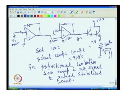
That means, if you see very closely if I set 100 degree, 100 degree if the set temperature is 100 degree; so if I take this you know the set temperature is 100 degree. Then, to maintain the assume that to maintain the oven at 100 degree c, the heater needs say 7 volt. The 7 volt here calls for 7 volt here calls for 8.2 volt here; 8.2 volt if you give only I get 7 volt. To get 8.2 volt if the gain is 1000 here, if the gain is given 1000 then I need
