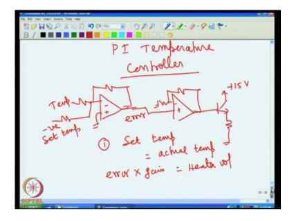
PI temperature controller - this actually gives much better performance than proportional controller so, this is extensively used. And we should understand why this integral action, PI - means proportional integral temperature controller. We also will see later, what is proportional integral differential temperature controller?
