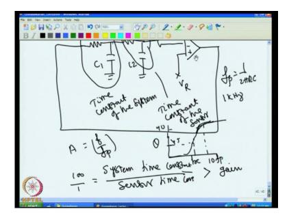
Now you can work out and see. I will show the gain for example, I find the system time constant divided by sensor time constant, I find the ratio between these two; then the
