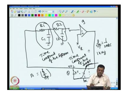
So if you do not want the loop to oscillate, we have to make sure either the phase shift is not 360 degree around the loop; or the gain is lower than what is attenuation provided by these two RC elements. If that is satisfied, then system cannot oscillate.
