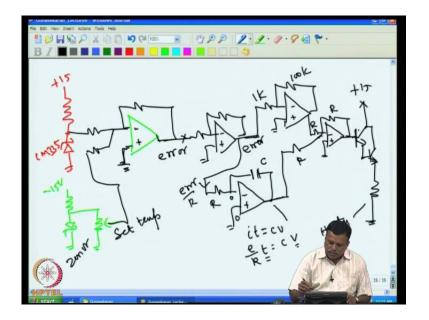
Suppose you may ask, what happens if the temperature had gone higher than the set value? Suppose, if the temperature goes higher than the set value - the error becomes minus; then the minus makes the reverse current flows that means - the capacitor will discharge and the voltage will reduce, and this voltage also will reduce. Anyway this minus actually become plus and this plus again become minus, so that again reduces this voltage.
