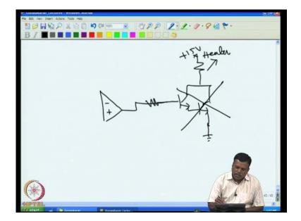
For example, if the heater voltage is 100 volt, if I connect the heater like this, I put a Darlington pair I will connect this one to ground, then connect the heater here plus 15 volt. This is heater and then this is our output driver, and the output of that is given to this of course there is series resistance.
