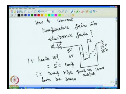
So, we should find out how to convert temperature gain to into electronic gain? Now for this, we had asked the question suppose, if I have a heater, how much voltage I have to give to raise the temperature of the oven by 1 degree? For example, if I take system like this, if I assume, this is the system and this is a heater, which was connected in our case
