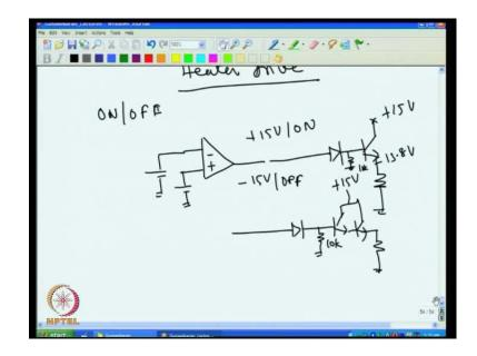
So, we will discuss about heater drive part. For on-off controller - first I can briefly explain for on-off controller - what is to be done? For on-off controller the heater either should be switched on or off.
