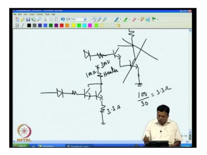
For example, I cannot have heater drive like this to drive a high voltage; for example, I cannot have this like what we have done in the on-off controller, so I can put this drive and I put this, for example, here plus 300 volt I put and then put this and then put this, this will not work, because what will happen is that if this voltage increases linearly.
