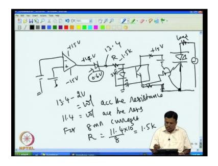
So, this is easier to handle or we can also use, for example, thyristor. So, in case of thyristor what we can do from this? We can have a drive and then we have to fire the thyristor; now, thyristor has to be isolated; the easiest way of doing this would be using a opto-isolator; for example, I can have the so whenever this is plus 15, then it will allows plus 15 to comes
