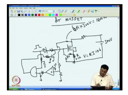
So, this work find for DC supply. In case, if want heater drive for the from heater drive from 230 volt AC, like if you want to use the triac and then control the heater particularly that is the very often use in i power over sense so on; so then using of this kind of triac this this kind of MOSFET or IGBT is not good, because you need DC voltage, of course, one can rectify the AC and give this.
