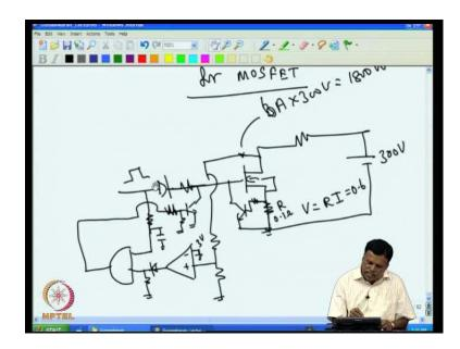
So, we should sends this and then switch of the drive itself, then only the MOSFET can be protected; so, what we do is, we at sense this one this one, so what we do is, next stage is you will sense this; this voltage, I can sense this by having a divider and see that what is the voltage if this is high compare to my reference, I put the reference here; for example, normally, if this will not be more than 3 volt circuit, so I keep here 3 volt, so the voltage goes more than 3 output will go high.
