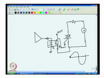
So, as the voltage increases more time it will be on and less time it will be off, that way power that is flowing is proportional to the error voltage; this way you can use the thyristor; only drawback of this circuit is, this ground must be equal to say this ground, then only current will flow through this; if you want to break this, we can add optoisolator for this circuit to make it such that, there is no shock hazard.
