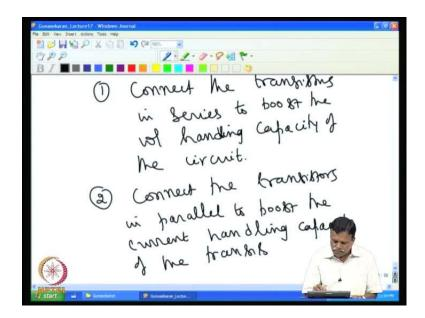
So, connect the transistors in series to boost the voltage and the capacity - voltage handling capacity - of the circuit. The individual transistors are still handling only low voltage, but now we can construct the circuit which can handle much higher voltage. Then, connect the transistors in parallel to boost the current handling capacity of the transistors or it can also be, that is, we can also say connect the transistors in series to reduce the heat dissipation transistors.
