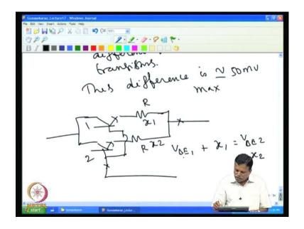
But then, if you look at the characteristics of the transistors, that base-emitter voltage, there will be difference, because for the same - current - collector current - what is the required base-emitter voltage for this and this? There will be a difference; the difference goes up to a maximum 50 millivolt. So, for the same current, for the same I c - collector current, V B E requirement is different for different transistors.
