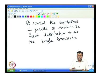
Connect the transistors in parallel to reduce the heat dissipation in one single transistor. This is essential to mainly see that the junction temperature is kept at the junction is kept at low temperature; that is why; we connect the transistors in parallel. So, one can connect the transistors in series or parallel without violating its working principle and then we can derive the advantage of increasing the power or increasing the voltage rating.
