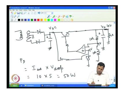
So, first let us take how to use the transistors in parallel; so, transistors in parallel. Because, if you want to increase the power capacity, then it is essential to increase the put the transistors in parallel. Let us take a typical linear power supply and then see how we can do this.
