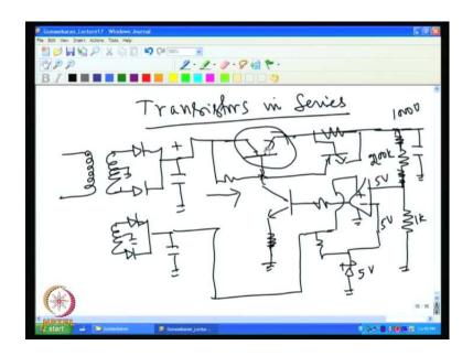
So, we may have to put normally about 250 volt that is what the normal resistor withstands. So, we may have to put per 1000 volt four resistors in series so that the voltage can be shared.
