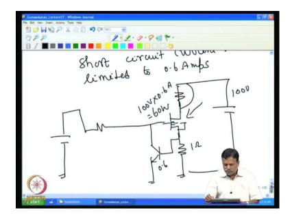
So, the current I comes as 0.6 amps. In this case, even if you are short circuit, current will not go beyond 0.6 ampere; so, short circuit current is limited to 0.6 ampere. Short circuit current is limited to 0.6 amps
