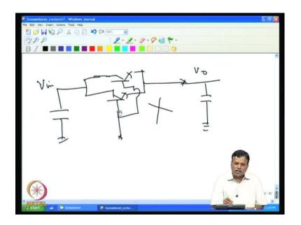
So, this is the essential point - that one not understand in connecting the transistors, without these two resistors, then current sharing will not be assured. This is because, if I connect them, for example, if I connect them directly in parallel without having the emitter resistance; then you have this arrangement. So, we put the V input here and then we get the V output (Refer Slide Time: 09.33).
