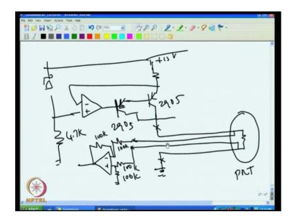
Now, this can be used further for controlling because this if we want to use it for control then, I have to find the error voltage. I take this and subtract with respect to reference temperature then I can get a difference and then I can do the same thing, which I have done the earlier that is in the case of thermocouple we are done. The same thing can be done I will not repeat this but, I am just concentrating on this sensor design.
