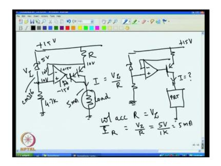
That is how the current is constant so even if I vary this current will remain constant but, actually how is the circuit is working? You know, using this mathematics if we look at how the circuit is working, we can approach this in a different way. Assume that you know, if this is 10 and if this is not 10 suppose, if this is more than 10 say 11 volt; suppose, if it goes more than 10 say 11 then this point will come down, because this is 10 and inverting input is 11.
