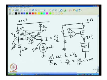
The base voltage output of the op amp have to change when temperature changes, whether output have to change say by 0.1 volt, the required difference change is a 0.1 divided by the open loop gain. The open loop gain is very high, so if the base emitter voltage changes with temperature then output voltage have to change by 0.1 volt or 0.2 volt then required change here, look at this is remaining 10 and the required change will be only few micro volts, because the gain is very large.
