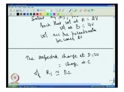
So, that means, the expected change at D will be again 2 volt, because C is changing by 2 volt so, D also expected to change 2 volt; so, next to this, the expected change at, that is, a change at D equal to 2 volt, that is, equal to change at C, and that is potentiometer change.
