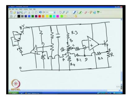
So, if D have to change by 2 volt then, if I take R 1 R 2 are equal, if R 1 equal to R 2, if R 1 is nearly equal to R 2, then, to get 2 volt change to get 2 volt change, to get 2 volt change here, if these are equal; we know that this point have to change to 4 volt, if 4 volt
