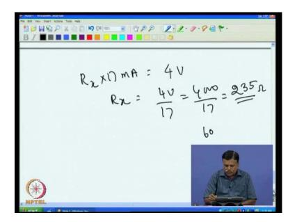
So, all the time to concentrate at this point, is that - how much resistance have to put to produce the 17 volt for 17 milliampere, 4 volt at 17 milliampere? So, the R x into 17 milliampere is supposed to give me roughly 4 volt, so that, you can find R x very easily by taking this; that actually, if you take this 34, you will have 6 3 9 0 so, you will get 2 for 35 ohms so, that is the approximately the resistance that is required for R x.
