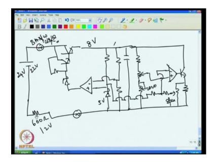
So, in practical usage, we find that there is no problem because of the noise; and we need not put too many wires because, the wires have to be long so, too many wires will cost more money and so, that problem all solved; and then, noise pickup is not there and even the small change in the voltage of this, and even load change or the wire resistance change also will have no effect on the signal here. That is how this 4-20 milliampere current transmitters are made, and it is used in the industry.
