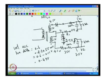
So, you will start from the LVDT. So, if this is LVDT primary and then two secondary voltages are here and the core is here, now I rectify this, then I join these two, then both are actually reverse connected. You have, this is here for, this, it is, sorry, for this the dot polarity, this is the dot polarity is here, this dot polarity is here. Essentially, when this is positive and at that time this is negative. So, that is what we wanted.
