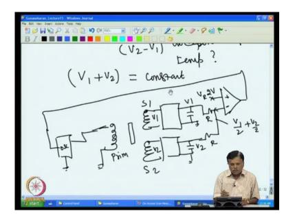
So, first step would be how to make, how to make V 2 minus V 1 independent of temperature, independent of temperature. Now, because of temperature the resistance of the wire changes, because of that we are getting error.
