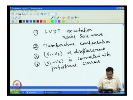
Today, we will continue the L V D T based position transmitter design and then see totality how this position transmitter looks like. So, far we are discussed about L V D T excitation that is we are shown how to excite the L V D T using sine wave. Then, we have discussed about temperature compensation for L V D T, then we are discussed about V 1 minus V 2 is proportional to displacement and then how to convert V 1 minus V 2 is converted into proportional current. (No audio from 01:25 to 01:32)
