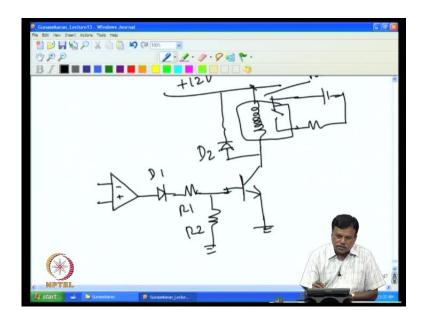
So, writing the problem statement actually what we want is, I will put a point here, I write here, it is when V output of op amp is plus 15 relay should be on, V output of op amp is minus 15 relay should be off. So, assume that we have given out that means how will you complete the circuit? I have to complete the circuit by linking the base to link this one to the base, so I put one diode plus I put one resistance here, so I call this is R 1 and this is R 2, you have two diodes D 1 and D 2.
