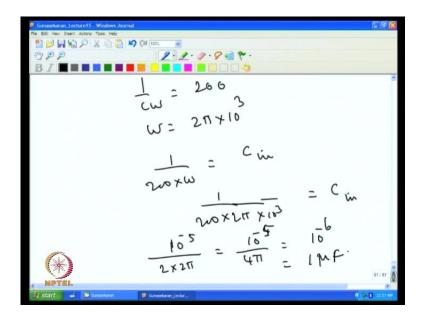
In this case, if you see this 2.2 k is dominant, because if we take 10 k and 18 k that is much higher than this 2.2 k. One can take roughly 2 k as the impedance of the input, impedance of the source, we take this is equivalent to 2 k so input impedance is 2 k. The capacitor should have much lower impedance than 2 k, so 10 times lower, I can take 1 by c omega should be 200 ohms 10 times lower. I had taken the omega is actually 2 pi into 10 power 3, 2 pi f at 1 kilo hertz.
