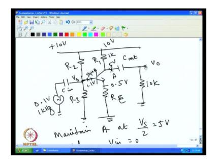
Now, we are very close to our design because we got the R 2, R 3 current and then voltage across R 3, that is, if you see the circuit, the voltage across R 3 is 1.1 volt and we know the current through this is 500 micro amps, then we can find out the value of R 3. Once, the value of R 3 is known, R 2 can be computed because we know the voltage
