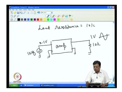
For example, what is the load that is supposed to be delivered to this amplified voltage? Load resistance just take it as 10 k; so, what we want is, we have to design amplifier using at transistor. So, I have this amplifier stage here and this input signal is given here; that is the input signal that is in 0.1 volt and then 1 kilo hertz the output is here, the output supposed to be loaded to 10 k; so 10 k I should get 1 volt a c supposed to come out, so how you go about designing this.
