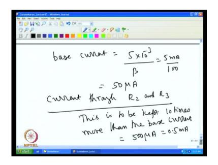
So I make current through now I find out current through the R 2 and R 3; this is what we decided this is to be kept 10 times more than the base current. We kept 10 times base current; actually it can be kept as 500 microamps or equal to 0.5 milliamps.
