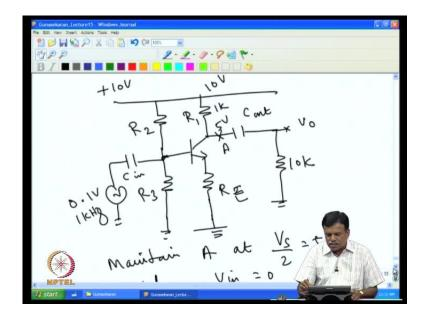
If this is a case, then now we have to fix the other two resistors that is - R 2 and R 3; that is R 2, R 3 this is two bias resistors, that is, these two bias resistors to be fixed.
