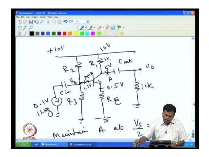
One can work out in the same line depending upon the supply voltage and the signal level and so on. One can always find to the same design, but one should be careful that when the voltage at the collector; if we for example, in this case, this amplifier works alright up to some point beyond which that it does not work. The limitation is that, if I
