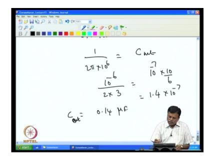
You will end up, 1 by c into 2 pi into 2 power 3 is equal to 10 power 3; so, you will have 1 by 2 pi into 10 power 6 as c coming in so that actually comes out to be 10 power minus 6 divided by 2 into roughly 3; so, 10 power minus 7 into 10 by 6 that is 1.4 into 10 power minus 7, which actually turns out to be. So, the c value comes out be c out rather, c out comes to be 0.14 micro farad.
