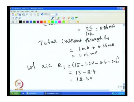
Voltage across R 1 is actually 15 minus 1.2 volt voltage across that is lost on the op amp minus 0.6 that is on the diode D 1 then minus 0.6 that is the base voltage; that is the voltage across the R 1 which works out to be 15 minus 2.4 that turns out to be 12.6 volt.
