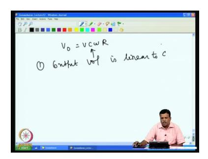
So, if you take the magnitude that actually comes as, the output voltage comes as V C omega R. That means the output voltage proportional to capacitance C, so output voltage is proportional to output voltage is linear to C linear to C.
