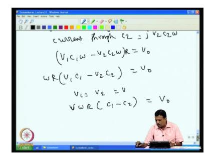
So, if you simplify this that it comes as we know V 1 C 1 minus V 2 C 2 into omega R. If we want equal to V 2, then we can write V 1 it is equal to V 2, because the minus in already consider. So, that makes it V 1 omega R, V into omega R equal to C 1 minus C 2. That actually becomes V naught but, then C 1 is coming because of one capacitor with respect d.
