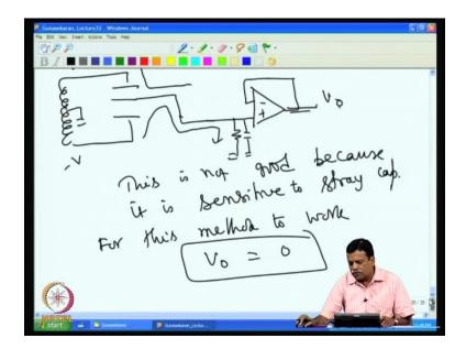
So, this is not good not good, because it is it is sensitive to stray capacitances stray caps. If this method has to be successful it should be a null method. So, this method, for this method to work, for this method to work method to work V naught should be equal to 0. This is very important actually otherwise, V naught is 0 then this capacitor because, V naught is 0 this voltage is 0 and this capacitor has no effect, then we have to modify the circuit just to make it V naught 0.
