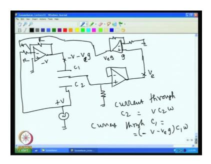
What can be done is, we can have the op amp circuit. Then for example, we can have this output then one of the plates for example, I can show like this, I have the source here, source I connect to this one plate and this I connect to this. Then, for bias current I put this resistance at the input then whatever voltage that output voltage I am getting that actually can be amplified. For example, I can have a amplifier here, I can amplify this
