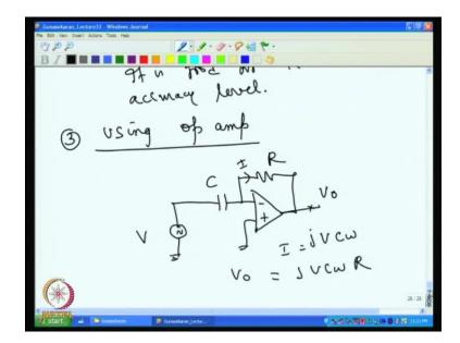
So, third technique at that what we going to discuss in detail would be, using operational amplifier. Now, if you want to measure the capacitance in operational amplifier, then one
