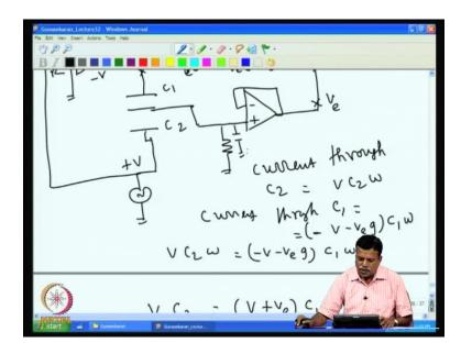
So, by this now if I write, then the bridge is getting balanced since, the bridge is getting balanced this capacitor is not a serious problem, the stray capacitor is not a serious problem, because the V e will be small if the gain is large.
