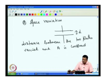
The second possibility is, space variation. That is we can have two capacitor plates. And keep the area same and vary the distance d, the distance between the two plates. So here, distance between the two plates are varied and keeping the area constant distance between the between the two plates varied and then A is kept constant. So, this is space variation can be also used.
