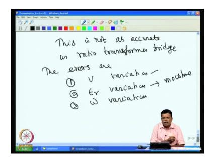
So this is not as accurate as ratio transformer bridge, as accurate as ratio transformer bridge. This is because, the errors are the errors are 1, V variation, epsilon r variation, omega variation. These are very serious problem because, the epsilon r can vary because of moisture can create problem and then source voltage can vary, frequency can vary. So
