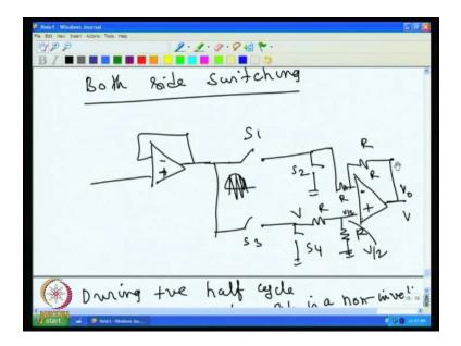
That is, what we do is, in the negative half cycle in the negative half cycle, I will keep this open and this is closed, so that you know the plus input is grounded, now S 3 is open. No signal is coming here and then, S 1 is on so, whatever signal is negative, signal is there to come here and S 2 is open, so that signal will be applied here and this is acting as a inverting amplifier.
