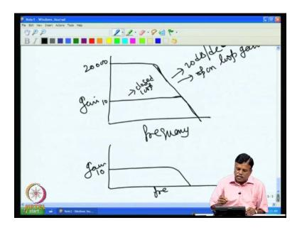
So the amplifiers, new amplifiers band width is like this; that is the gain. This is frequency if we plot; that you get that is the amplifiers band width that is, the D C is the gain 10.
