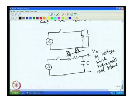
So, I can do in the following manner, instead of having the load like this. I can have a switch, then I can put one R C like this. Now at this point, you will have signal plus noise that is coming here. At this point, if I see that is v 0 then, this is a capacitor use to average out, at this point I will have D C voltage which represent only signal.
