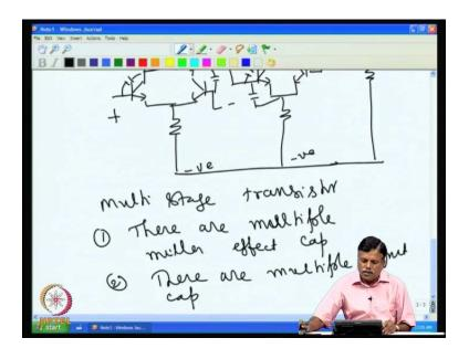
The multi stage transistor amplifier has multiple poles and zero that is the worry, because for example, if we take this, that we have a capacitor from here to here and then you also have a capacitor from here to here and so on, that all the stages have their own miller capacitances and then also you have this and then also the you have the input capacitances also there, which limits the low frequency performance.
