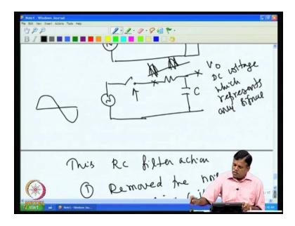
So, this noise ejection happens, only if the switching is done correctly, because this should be on during the positive half cycle and it should be off during the negative off cycle then, the averaging can take then only averaging can take place. One should find
