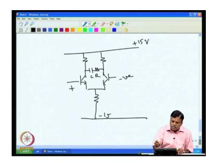
So normally, the manufacturers do the frequency compensation inside the operation amplifier itself so that, the amplifier is stable and then it works as a amplifier. That is done invariably in the first stage by adding a R C at this point, so we have plus here and then the minus input and the plus supply plus 15 volt supply here.
