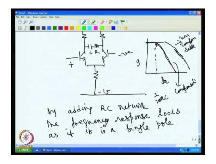
The open loop gain is drastically reduced, we are achieved this stability by drastically reducing the overall open loop gain of the amplifier. The dominant pole compensation is good, we look at the positive part of it.
