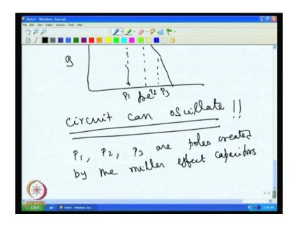
The reason is that, in the here is a pole, this is created by one R C component mostly it is actually, miller effect capacitor and the resistance also associated that. So, miller effect capacitor first stage and the resistance associated with the input can create a this pole one and then you have the second pole here, P 2 and third pole here, P 3 so, P 1, P 2, P 3 are poles created created by the miller effect capacitors. P 1, P 2, P 3 are poles created by the miller effect capacitors.
