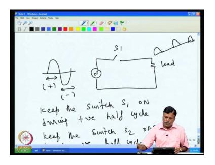
Now, how will you achieve this? Now, one can do this in the following manner; assume that we have a sine wave that is we have input sine wave like this. Then, we will have switch here, then I operate the switch. Switch is on, that is this is positive half cycle, we have positive half cycle and this is a negative half cycle so, this is a positive and this a negative half cycle. Keep the switch on that is, keep the switch on switch S 1 on during positive half cycle.
