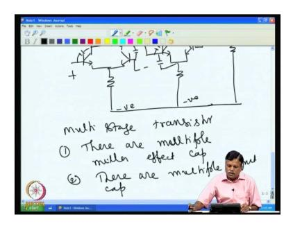
Now, that is there are multiple there are multiple multiple miller effect capacitors miller effect capacitors .Similarly, there are multiple input input capacitors input cap and the
