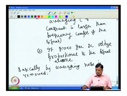
So, the by averaging technique, one can remove the noise. Basically, lock-in amplifier works by averaging that noise is removed. So, basically by averaging noise is removed. So, this is a basic working principle of the lock-in amplifier.
