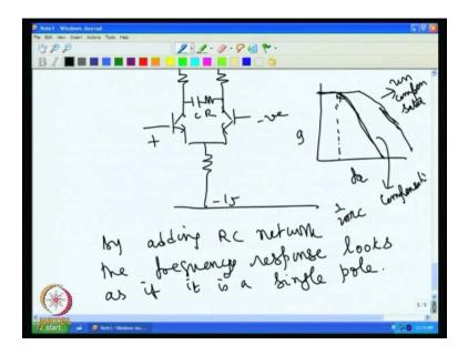
Is that, it is very stable. You can depend on this. It will never oscillate but, the bad part of if it is the open loop gain is drastically reduced, open loop gain is reduced drastically. So, the frequency open loop gain is drastically reduced except at, low frequency that, it all I if we look at high frequency, the gain is drastically reduced. This is the bad part of it
