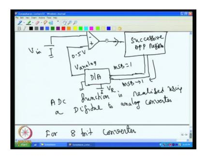
So DAC puts a 0.5 volt and the output of the DAC now it is become 0.5 volt. So, if this is MSB is 1 and the output here is 0.5 volt. So, the successive approximation starts the its operation by output in MSB alone 1 and all other bits are too zero so if we have MSB alone 1 and then the DTA converter responder putting 0.5 volt.
