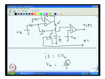
So how to improve because the drawback here is suppose C changes with temperature and then even the change in the resistance with temperature all will give error because, if C changes then we see that the C is a parameter in the equation, so we are just measuring t so if we are measuring only t then, we at make sure that this i and C is constant, but, both i as well as C can change with respect to temperature.
