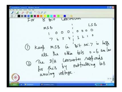
Now, the converter works like this that is you know here, if we have a for example, for 8 bit converter we take an example for say for 8 bit converter what we do is we 1st put that 8 bit converter means that we will have 8 bits are there so we will have MSB here and then we have a LSB least significant bit here so assume that we have a 8 bits so, I do is I will have, so in this case I take this is the lower 4 bits and this is the higher 4 bits.
