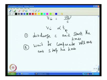
So, in this method start this discharge C and start the timer, then after that the second step would be wait for comparator roll over and stop the timer, so the time can be measured that gives you V in, but, if we see both the methods both are them are not really matching with the dual slope comparator we have discussed earlier.
