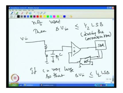
Then V input change delta V in change during the conversion should be less than half LSB. It must be less than half LSB then 1 need not uses the sample and hold now sometimes people do is trick that you know, you can have the input voltages coming that for example, if I have a V input if I am dividing the resistance and if I have a very large capacitor here then this can be given to for example, this has go to our ADC, it can be used ADC output.
