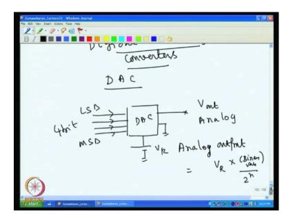
So, general block diagram would be that we have digital input are given for example, 4 bit converter 4 bit converter we have a L S B here M S B here there the input 0's and 1's and D T A converter and this as the reference voltage V reference and then we get analog output V output analog.
