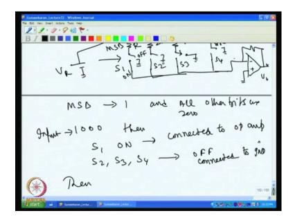
So, what happening is when M S B is high, when M S B is 1 and all others are 0, it is 0 by that is we have a condition for 1 0 0 0 input input is 1 0 0 0 then we call that is S 1 S 2 S 3 S 4 then S 1 on then S 2 S 3 S 4 off; then this actually given to V reference is given to V reference then then S 1 on S 1 this is off position this is on position on position connected to connected to op amp this all connected to ground all connected to ground connected to ground.
