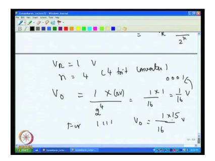
For example, if it is a 4 bit convertor then it is a 1 volt V reference equal to say 1 volt and n is equal to 4, 4 bit converter then analog output V 0 would be equal to 1 volt into 2 power 4 that is actually into binary value. So, that will be 1 by 16 into for example, if 1 L S B alone on as I if you have a logic 0 0 0 1 for this then the final value is 1, then you have 1 by 16 th of volt.
