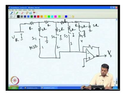
Now, let us see how the convertor is fabricated using this R 2 R technique. So, here what is done is that you have the resistors R 2 R is put, then you had the same summing amplifier, I can have this, then we can have the next this is R and then 2 R this is R and then we have next bit can activate this, then third bit and then the forth bit. So, this is M S B 1 2 3 4 and the last one 2 R. So, this is 2 R and then R and then 2 R here 2 R.
