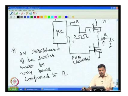
So, because of this this is may not be accurate one way of improving this would be can have switches connect at the p w m output, we have a micro controller and then plus 5 volt the p w m output output can be suitably scaled using the fetch switches at the output for example, we can have fetch switches and this can be connected to a V reference, which may be say 1 volt and this can have 5 volt logic.
