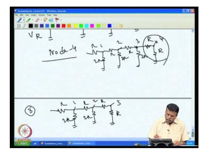
Now, if I simplify this you can have next that is that is simplified up to node 3, so this up to node 4, so I have simplified up to node 3 now, you have R here 2 R then, I can make this R 2 R third one, I can show this is R and then I can write it as R, this is node 3; because if you see this, this 2 constitute 2 R and that parallel to 2 R that makes is it R. So, you have R 2 R this is node 1 and this is node 2, that becomes a node 3.
