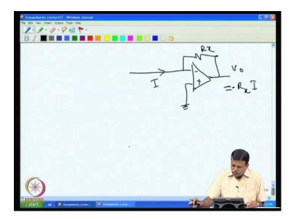
Then the final output voltage and the output of the op amp, because we have used the summing amplifier op amp is summing amplifier. So, all the current whatever is coming is actually pass through the resistance R x. So, you have I here coming here that is output voltage that is equal to R x into I with minus input.
