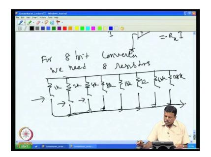
Then, for 8 bit converter for 8 bit converter, we need 8 resistors that is we need actually the same we need the same 8 resistors, if you look at this 8 resistors the accuracy demanded automatically goes high, because we connect we connect join all of them we join all of them and then, so we will have for example, 1 k 2 k 4 k that will be 8 k 16 k 32 k 64 k 128 k and then, this is the output current that is a digital word is switching each one separately.
