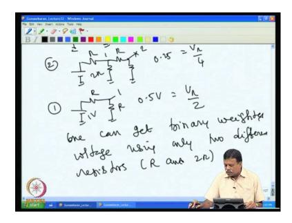
So, one can get one can get binary weighted voltage binary weighted voltage using only two different resistors, this R and 2 R. So, this easier to fabricate R only 2 resistors with high accuracy that is why, this can type of convertor is a very popular.
