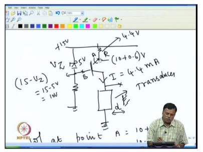
So, that comes out to be 0.6 minus 2.2 into 55 into 10 power minus 3, that comes 0.6 minus 2.2 into 55 that comes out to be 55 into 2. 2, that comes out to be 121 milli volt that is 0.6 minus point 1.2 that will be 0.48 volt so V B E at 100 degree c would be 0.48 volt. So that, makes what is the voltage at point A, because this voltage at b is at 10 volt and voltage at B is at 10 volt and then V B E is 0.48 then A will be 10.48 volt so voltage at A will 10.48 volt.
