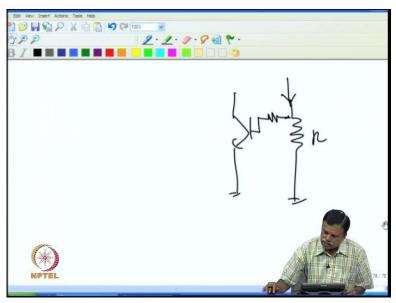
So, this is a series which because if I connect directly the R 2 T 2 then you do not get that benefit for example, if I connect like this so I have resistance here, and this is R and if the current is flowing through this, and if I connect directly the transistor here to switch on. Now, at room temperature what is required the voltage difference required is 0.6 volt.
