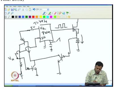
So, what I do is for example, I put the switch here then I have take this I connect to transistor here for example, to switch, and if I take for example, P M W I C as T 1 494 we have and this one has a reference output V reference a 5 volt is available. So, I can connect this 5 volt through transistor and this can be connected to this. So, when the current goes high here, then this transistor will be switched on once this transistor on whatever emitter current that will flow through this.
