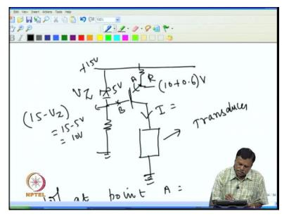
So, voltage at I call this is the point a, this is A, so voltage at point A is assume this is a zener voltage at point A we had find out. So, this is zener voltage assume this is 5 volt, this will be is not zener voltage actually this voltage at this point is I call it as B. So, voltage at this point will be 15 minus V Z, because this is 15 and voltage across is 5 voltage at this point will be 15 minus V Z that will be 15 minus 5 that will be 10 volt.
