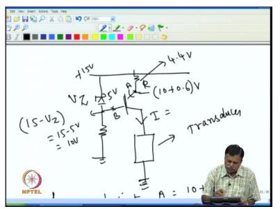
So, we got the voltage across this resistance R has 4.4 volt, so we know that base current is negligible then voltage across this is known and if I know the resistance value then I know the current flowing through this. So, assuming R has 1 k, if R is 1 k if R equal to 1 k then current through R would be that is this resistance we had find out current through this R. So, voltage across is 4.4 and the resistance value is 1 k, so if I take 1 k then current through R would be 4.4 milli ampere.
