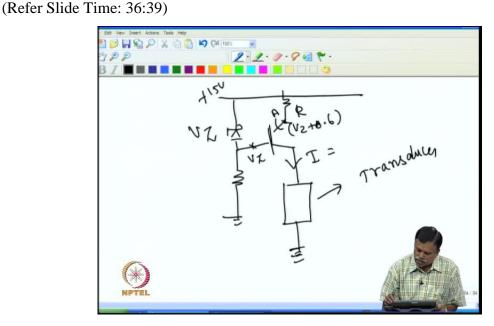
For example, I put the circuit like this. So, you have a transducer, transistor assume this is supply voltage then I have a (()) diode connected this then I have the resistance here for example, this is plus 15 volt and then this is a load. If I take this load can be now transducer, this can be a transducer essentially there is a current that is flowing through this transducer. because this is I, I is nothing but this is V Z this is R. So, if this is V Z we
