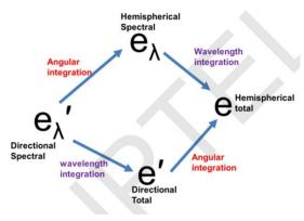
To arrive at more practical forms used in applications like Earth's energy balance, two types of integration are carried out:
