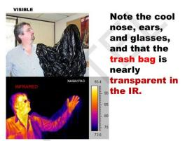
The distinction between a body that appears black in color and a true blackbody is important. A body that is black in color in the visible spectrum does not necessarily absorb all radiation across all wavelengths. For example, a plastic sheet that appears
