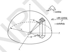
The solid angle is a key concept in radiation because photons are emitted in all directions, covering  $4\pi$  steradians. For example, photons can be emitted perpendicular to the surface or at other zenith angles ( $\theta$ ) and azimuthal angles ( $\varphi$ ). It is essential to define the radiation emitted for each angle, both zenith and azimuth.
