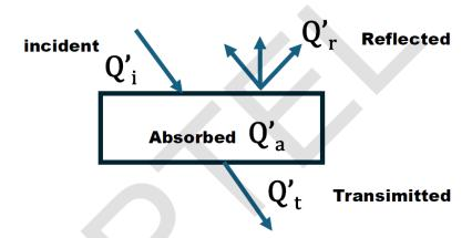
Relation between reflected , transmitted and absorbed radiation
