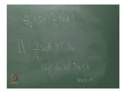
And you try to figure out what the outgoing angle is let us say I do sin inverse n 1 over n 2 sin theta 1 if it turns out that n 1 is greater than n 2 and its significantly greater and let us say this sin theta one ends up being significantly large is not it possible inside of here to get a value greater than 1 does that mean Snell's law is wrong the way I mean it has to cant violate the laws of trigonometry right so.
