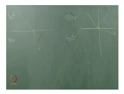
So, if I have a fast material and a slow material and the light ray is coming down going to make it look like it is about 45 degrees, what should happen to it? The waves are going to be propagating more slowly in the slow material. So, that causes it to bend upward or downward is that right down or up.
