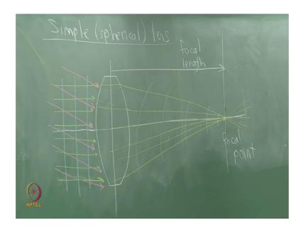
You ever have a bad straight line day you know also. So, so what is going to happen is in this lens is that we effect of refraction is going to cause these rays to bend inward to start to converge and if we make a simple spherical lens they will converge to a point somewhere.
