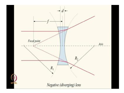
So, there is also diverging lenses if you seen optics before it should not be surprising. So, there is a diverging case where we can make rays of light instead of converging spread apart and I will just mention the sign convention in this case. So, R 1 in this case is less than 0 and R 2 is greater than 0 and so, you can directly apply the lens maker's equation in the original form and in the thin lens approximation to determine the focal point.
