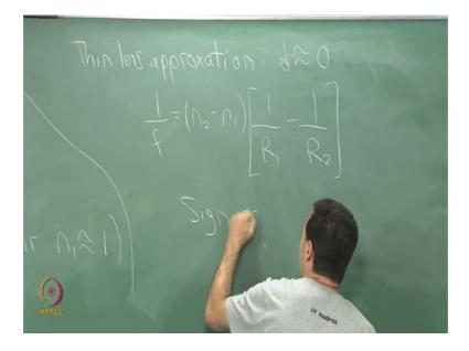
So, this is the index of refraction for the lens material there is a simple approximation that is often used to this and I will write that here it is called the thin lens approximation this is much more common now after this approximation where we get rid of this d parameter. So, here we say d is approximately equal to 0 in which case the lens maker's equation simplifies to 1 over f equals n 2 minus n 1.
