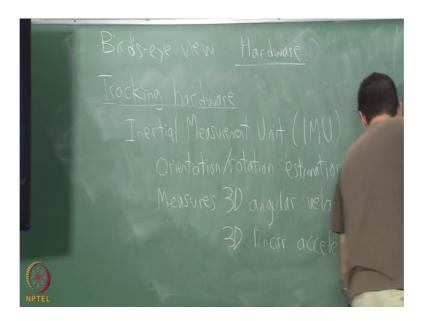
Tracking so, you call this tracking or estimation or filtering. So, people in electrical engineering will tend to use words more like that. One of the most useful components is the inertial measurement unit people call it IMU.
