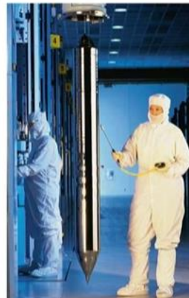
Wafers are cut from boules , which are large logs of uniform silicon.
