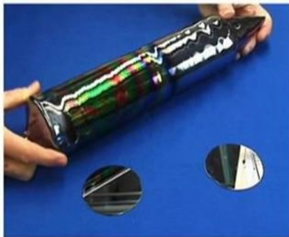
Wafers are cut from boules , which are large logs of uniform silicon.
