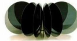
4. Wafers ready for processing – 4 to 12 inch diameter are standard
