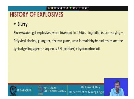
And, as we have discussed the ammonium nitrate ammonium nitrate is also used as slurry explosive, where ingredients are the polyvinyl alcohol guargum, dextran gums, urea formaldehyde, resins etcetera. These are used mixed each other and it along with the hydrocarbon oils, ammonium nitrate; ammonium nitrate is essentially required because it is the oxidizer it is the main source of energy.
