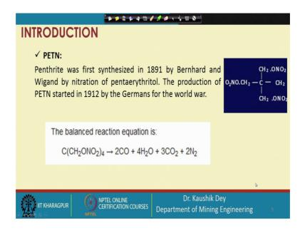
And, on inquiry of that people learnt that the ammonium nitrate may be a very very suitable explosive if it is used as the explosive material. So, from that invention in 1955 onward ammonium nitrate the developed in a prill form and mixing that prilled
