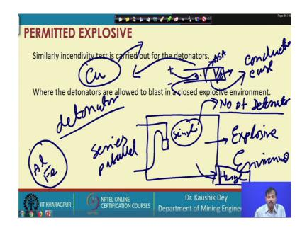
Similarly, incendivity test is carried out; incendivity test is carried out for the detonator, where the detonators are allowed to blast in a closed explosive environment.
