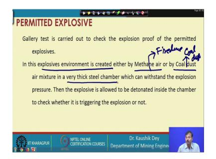
So, gallery test is carried out to check the explosion proof of the permitted explosive. In this explosive in this case explosive environment is created either by methane air or by coal dust air mixture in a very thick steel chamber.
