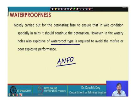
So, next one is the waterproofness. The mostly waterproofness is carried out for the detonating fuse and to ensure that in wet condition also specially in rain, it should continue the detonation. So, there is no chance of cutoff the of the detonation in between
