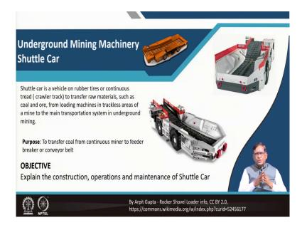
Now, like we told about this your rocker shovel, a very old machine, this mining machinery this particular type of machinery is also a very old machine. It started even I think in 1880's also, this type of machines were used and then, it developed over the years. Now, today is the modern shuttle car, which is manufactured by many companies like Joy or the Sandvik or Caterpillar.
