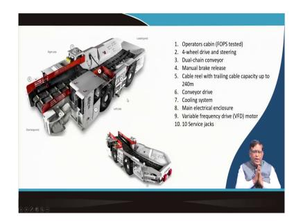
Now, in this figure, you can see the different component in a much clearer way. So, that means, this machines as a operator cabin is there, you can see this operator cabin it is located, which is ergonomically designed, a modern of machines has got a very good that comfortable positions and it is all the levers and all are very easy to operate, he can work in a dust free, noise free surrounding inside this cab.
