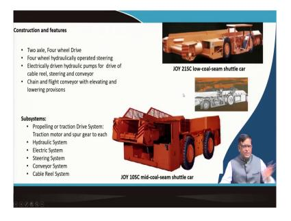
So, coming to this construction wise as you can see from that figure this is a from the figure, once very old shuttle car is also shown over here that is a it is a comparatively that before the previous figure, this figure is a very low height, here is a medium height, there we can have the operator can be sitting by the side of it.
