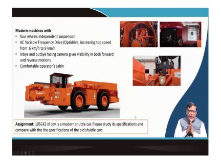
Then, that a lot of development have taken place to this 1880 model. In 1980, when this our variable frequency drive was introduced after that, all the shuttle cars which are being manufactured today are all having advanced feature. Now, there is a first thing was the development came with the suspension systems.
