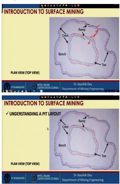
So, now, we can see in this layout also this is a simple hand sketch, which is showing a circular pit of portion, here you can see this is the ramp, this is the higher elevation, this is the lower elevation, this is the higher elevation, these elevations are the same elevation. So, this is the bench width, this is bench height, and you can have this as the lower bench. So, this is the bench, this is the crest line, this is the ramp, and this is the toe.
