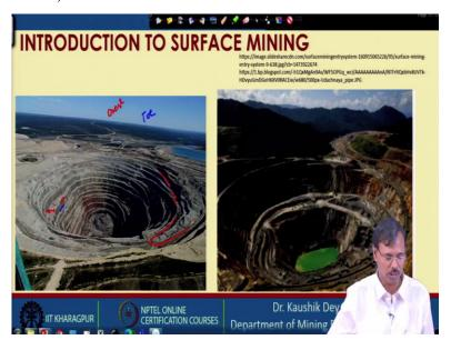
And if you look into this, you can see these are the circular pits you can see these are the benches you can see this is the bench. This is the crest line, this is the toe line, so toe, crest. So, similarly, you can see, and these are the ramps. You can see these are the ramps showing in the mine layout.
