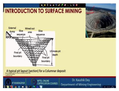
This is for the Columnar deposit, how it can be carried out this is a simple example of this one you can see the outside dumping is carried out in this case also this is the outside dumps placed at this position.
