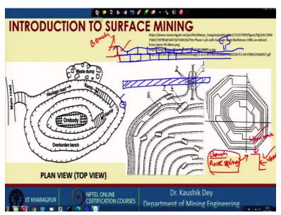
So, as we have covered the stripping ratio, we will directly start with the mining layout in this lecture. This is the most common layout which is practised in mining. So, this view is basically the plan view or top view. Now, let us understand the way we go for swaying the layout. You see, there is a line having some dotted line towards the insight. This is basically showing us the phases of the phase of mining working. How is it described? Let me show you the plan and sectional view.
