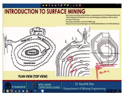
This is called ramp, which means you are coming through this ramp from this level to this level. So, similar way, you can draw it like this. So, this is crest line, this is also crest line, and this is showing the ramp because it is elevation here elevation is less. So, this is called a ramp, and you can clearly understand this ramp is going from here to here. You can see in this case,
