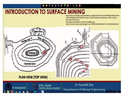
Let me clear it once again you see, in this case, this elevation is higher. So, this elevation is higher. This elevation is lower. So that means your ramp is on this side. Here, this is upper elevation. This is lower elevation so this is like this again, this is moving like this. So, this is the general technique to construct the layout of a mine, and you see, in this case, this is this one.
