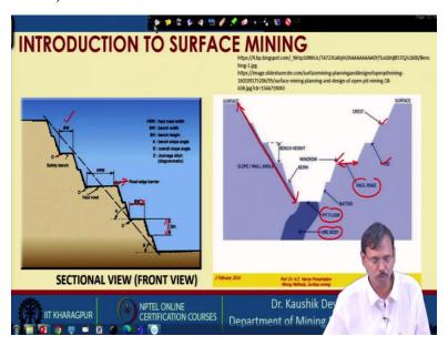
So, this is the typical terminology for a bench. So, this is called bench width, this is drainage provided or ditch provided. This is the safety bond provided so that the trucks, etcetera, will not topple down to the lower bench and this is the bench height, this is the bench width. This is the general terminology. This is called pit floor. This is orebody, this is haul road you can see the wider bench width is provided, this is the berm, this is a crest, this toe and this is bench height.
