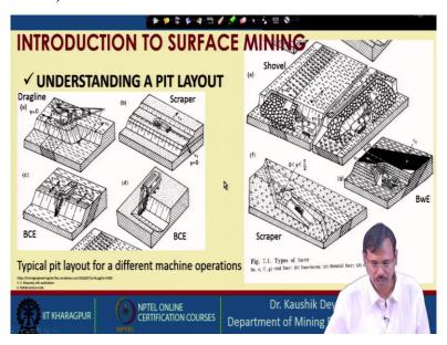
This is the layout for the operation of different machines, draglines, scrapper, bucket chain excavator, shovel, so these are the different layouts. So, this is more or less about the layout of the surface mines, how we will position, how we will position the machines, how the different terminologies are expressed, and how the mine plan is how it is sewing is shown in this lecture. So, let us stop this lecture at this position, will discuss the phases of mining in the next class. Thank you.
