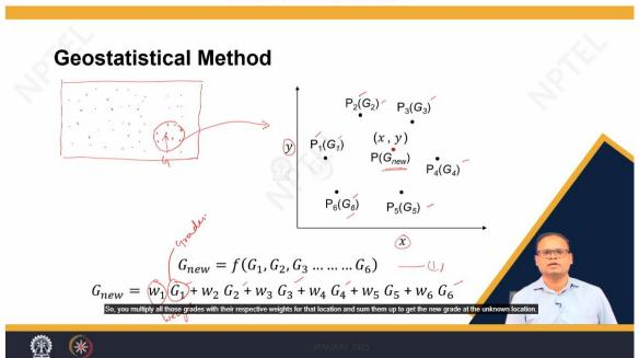
after D. G. Krige, is a mathematical procedure for assigning linear weights to samples to estimate grades at unknown locations.
