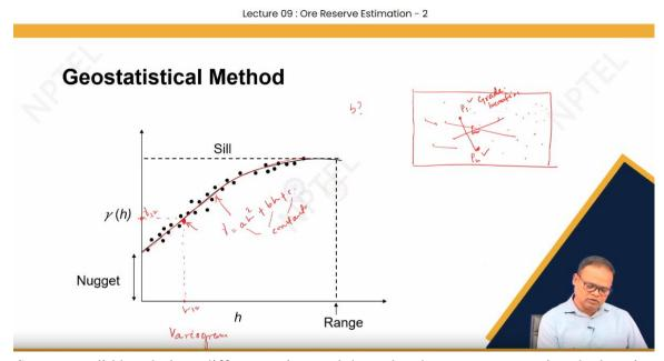
So, we we did borehole at different points and these dots here are representing the location of the boreholes. and we know ah you know what what are the grades at these ah you know borehole locations ah. For example, you know this is a point let us say this is  $p_1$  and this is
