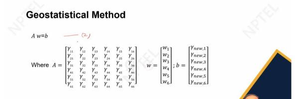
So, the previous equation can also be represented in matrix form as Equation 2 here, which is A matrix multiplied by W matrix equals B matrix, where A matrix is called a varianc
