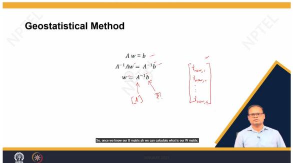
So, you calculate what is the variance matrix A. So, this is the first step of this the geostatistical method here. And this equation you know once we know that A matrix into W matrix is our B matrix. So, here what we can do we can multiply A inverse in both the sides. So, A inverse into A ah becomes you know A inverse into ah A inverse into A ah into W matrix becomes ah A inverse into B matrix B matrix yes. So, or we can write ah you know W matrix equal to A inverse into
