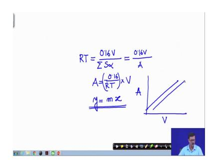
So, it is the RT, RT is equal to 0.16 V S alpha which is summation. So, this is the total absorption. So, I write capital A and this is 0.16 V.
