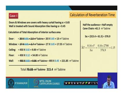
So, I have first case as I will do some covering, I will cover the door and window by heavy curtains having alpha value 0.65. And the wall be treated with the absorption some absorptive tiles having alpha point. So, I have taken this two decision, I will treat the wall and I will treat the door and window by virtue of some the curtains.
