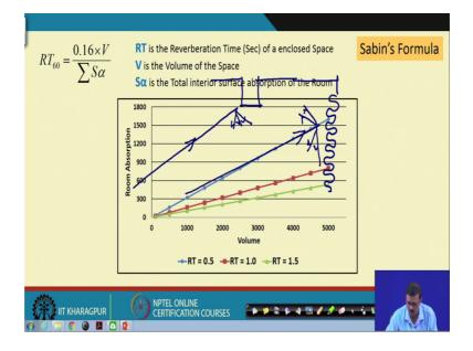
So, here let us again go back to the Sabine's equation, which is given as you know that RT is equal to 0.16 V by S alpha, I have put a summation sign because, it is summation of the S alpha the sum of the various surfaces and it is product of the it is the absorption coefficient.
