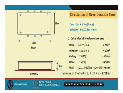
So, let us next stage let us try to calculate the how the reverberation time can be calculate what are the steps what are the formulations. So, I have drawn a plan of a hall of 30 meter by 15 meter and, the height of the hall is 6 meter which is given in the section and this hall is having 4 doors of 2 meter by 2.5 meter and 3 meter by 1.5 meter 6 windows which is plotted in this plan in blue colour.
