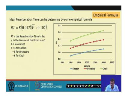
Next let us go to the another empirical formula, where the RT can be calculated by virtue of some volume. So, after this Sabine's equation lot of physicist actually go into calculate the RT and, this RT value is not going to be fixed for same, I mean different type of performance will be required different type of RT.
