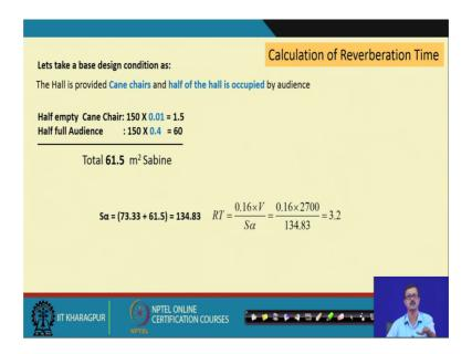
Now, let us take a design based case, I am going to design this particular room for a base case, where I have going to use the cane chair and, the half the hall is occupied so; that means, the half the hall will be occupied and rest half is cane chair and, this will be my best design condition and for that I want to set up a particular the design the RT value.
