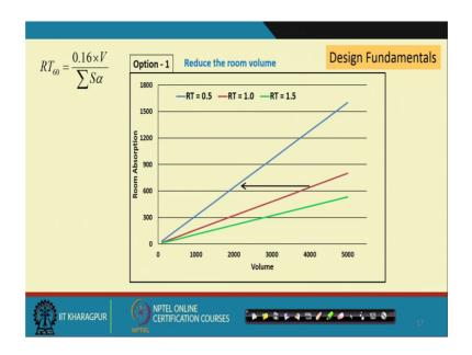
Now, there are way to handle this particular scenario, am I understanding is that I being a designer being a acoustical designer, I have to provide some RT, or some design RT for a particular room and, when I got a particular room or a hall, it is all reflective surface plastered surface and all reflective surface. So, I have to render it with some different material and finally, I have to propose the material and finally, I have to give some kind of the RT I mean achieve some RT value.
